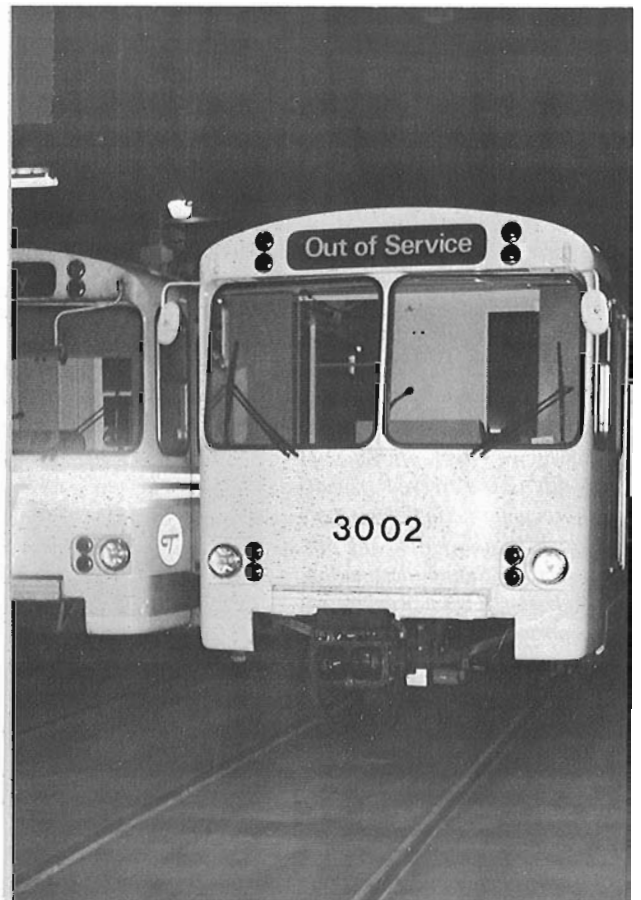
Experimental Car No. 3002, fitted with A.C. traction motors, was seen skulking in the back of the Anderson Road storage barns.
