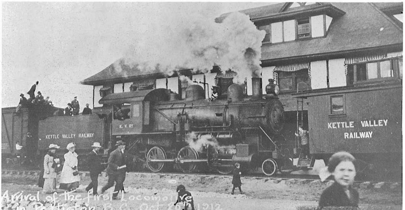
This historic photo shows the arrival of the first locomotive at Pentiction on October 26, 1912. The KVR purchased the 2-6-0 from the Chicago Iron Works, a second hand locomotive dealer, in July 1912. The locomotive and related railway equipment were brought to Pentiction by barge over Lake Okanagan. This permitted the KVR to open a third front for construction purposes.
