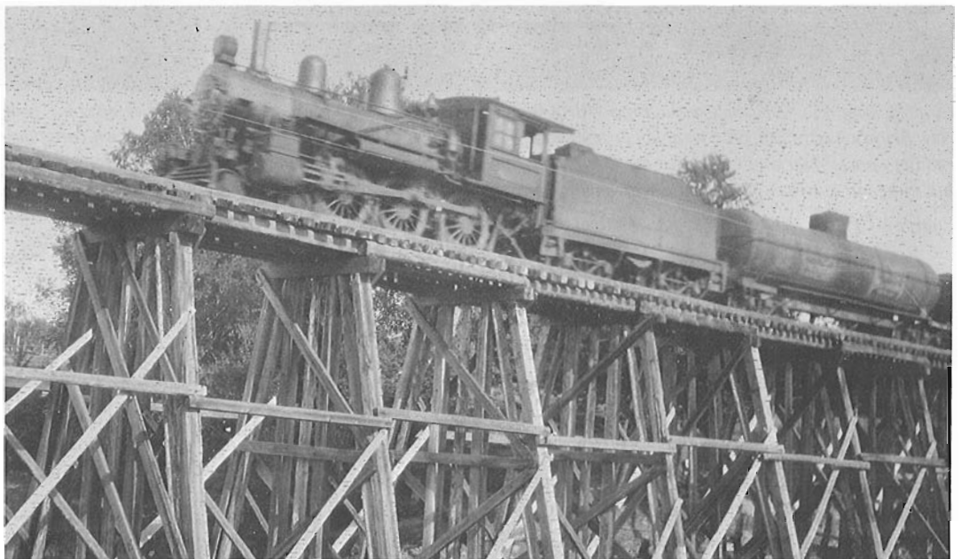
While this is a less than crisp view, it is the only picture of a Quebec Oriental locomotive which your co-editor has been able to locate. This picture shows locomotive 16 on the trestle at Black Capes, a point slightly east of New Richmond. The 4-6-0 was built by the Montreal Locomotive Works and was one of the engines acquired by CN when it took over the railway. Assigned CN number 1200 for corporate purposes, the number was never applied to the engine as it was retired shortly after CN took over the line in 1929.
