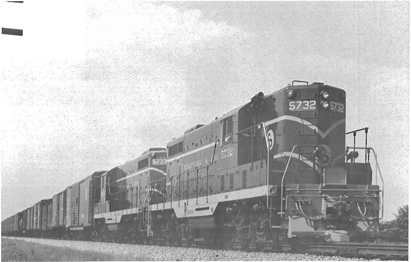
Heading a manifest freight, Canadian built GP-7's 5732 and 5733 head east out of Windsor in this June 1952 view. The Chesapeake & Ohio, one of the predecessors of today's owner CSX, purchased the diesel fleet assigned to its Canadian lines from General Motors Diesel Division plant in London, Ontario in order to avoid paying duties on U.S. built power.
