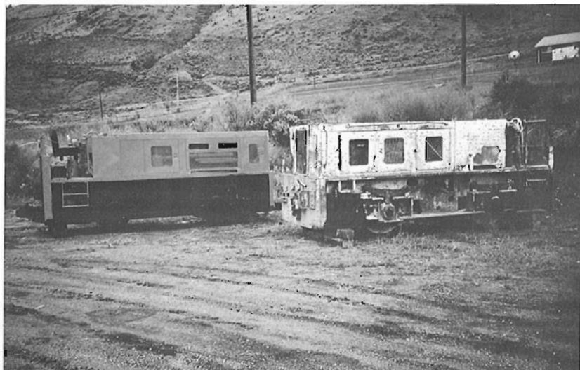
Two Plymouth JMD24 36" gauge 25 ton diesel-mechanical units sit in the yard of Nelmaco, in Savona in September 1989, waiting for road transportation to their new owners in Kemano and Minneapolis.
