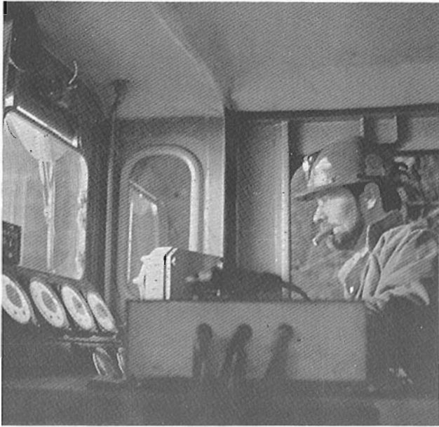
Inside the engineer's cab of one of the 42" gauge Mitsubishi 750 horsepower double-ended electric locomotives used on the run between Tide Lake and the Granduc Mine, about 1971 Photo from Granduc Operating Co.
