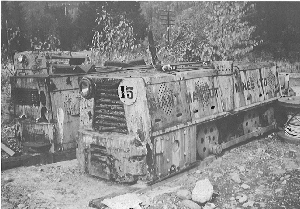
Parked in the dealer's yard in Hope, in August 1989, are three 4-wheeled locomotives (from right to left): North British built 30" gauge 15 ton unit number 15, Plymouth-built unnumbered unit with locally-made protective steel cover, also one of the Ruston & Hornsby units. All came from the Giant Mascot Mines Ltd. operation to the northwest of here.
