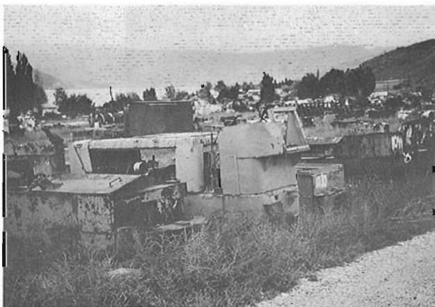
Nelmaco's yard in Savona, showing the variety of rail stock stored there. In front (from left to right) are: 4-wheel battery-electric unit, 4-wheel diesel-mechanical unit, another 4-wheel battery unit, then two steel ore cars.
