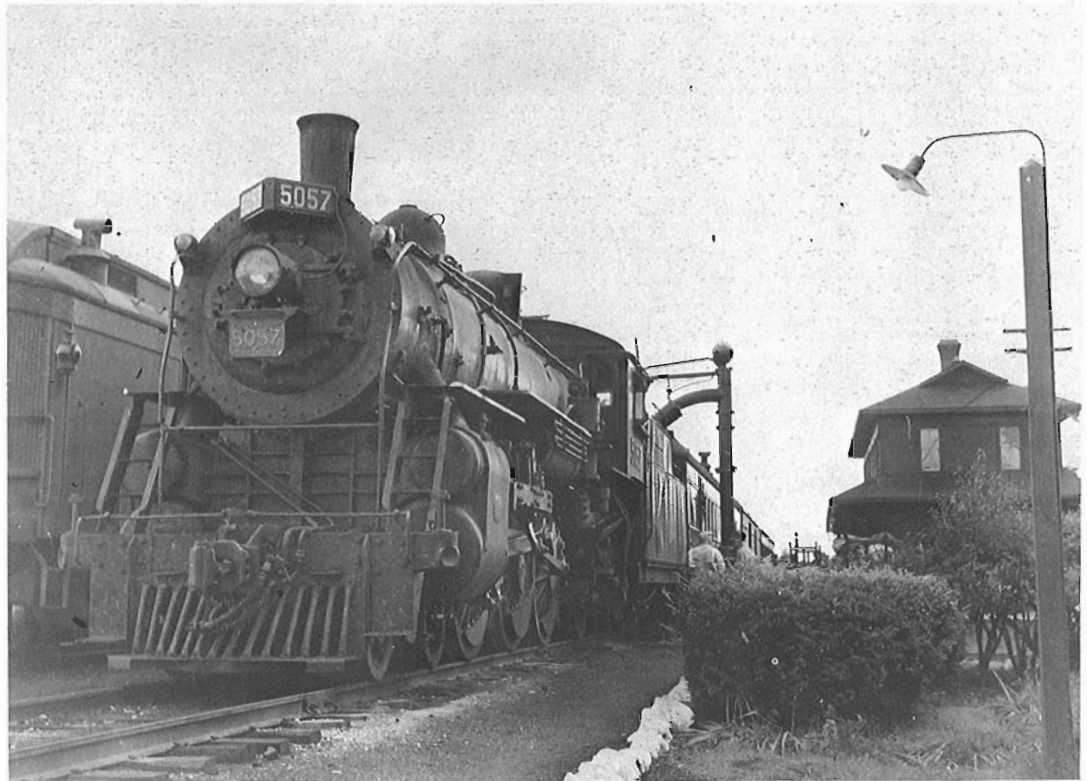
CN Pacific 5057 stands at the Lindsay station with a three car train. While the fireman uses the opportunity to replenish the water supply in the tender, mail, baggage, express and passengers have been discharged and loaded. After a scheduled ten minute station stop, the train will start on the final leg of its Toronto to Peterborough trip. Source: Paterson-George Collection.
