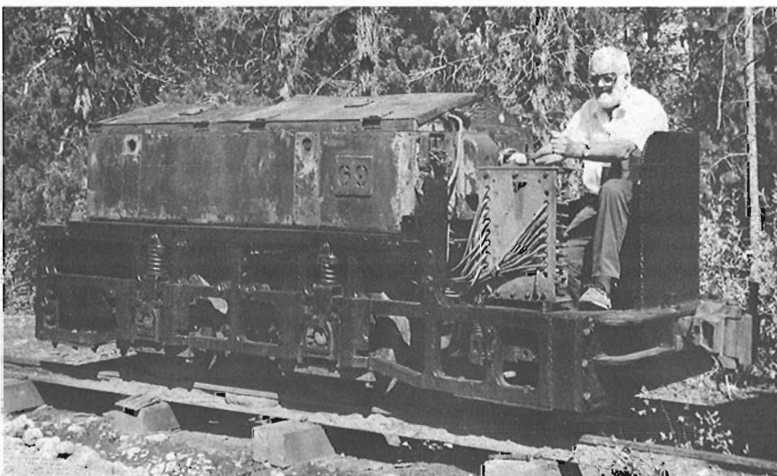
Cominco 36" gauge battery-electric locomotive number 69 sits in the Happy Hans Campground in Kimberley, in September 1989, with a variety of mining stock from the nearby Sullivan Mine.
