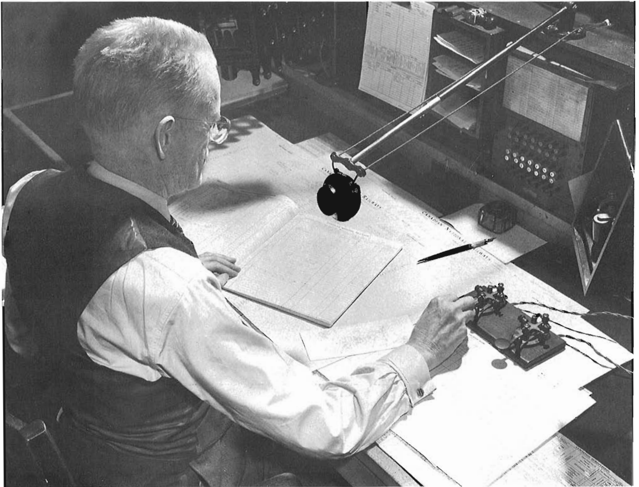
This photo of a Montreal train dispatcher was taken about 1950. Note the solid telephone transmitter arm and dual telegraph key. The train sheets, train order book and the blotter are timeless now. Note the selector box with the buttons to call individual stations.
