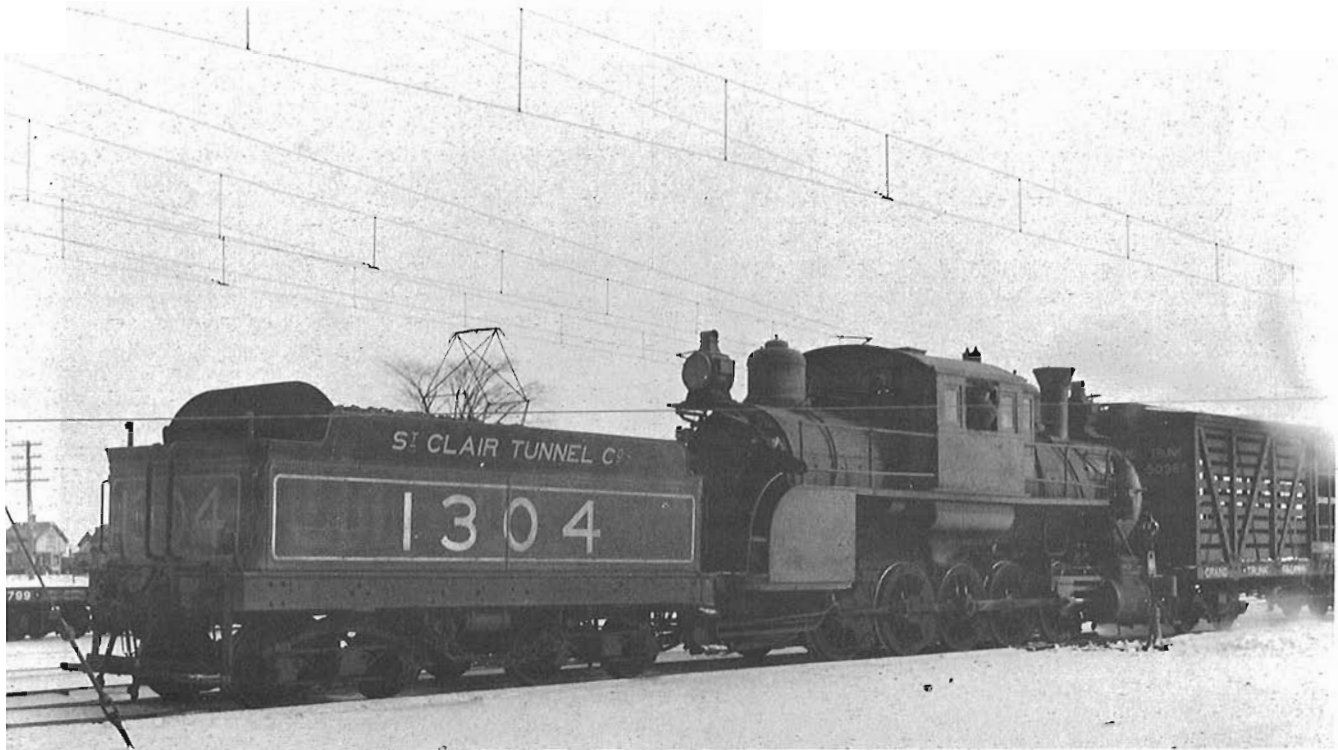
The modification of the tunnel locomotives from tank to tender equipped locomotives did not improve their aesthetics. This view, which was taken in 1908, shows the large firebox which challenged the fireman. Originally numbered 598 to 601, the quartet of tunnel locomotives were renumbered 1301 to 1304 in 1898. These units remained in yard service after being displaced from tunnel service. The first unit was retired in 1916 and the other three in 1920.
