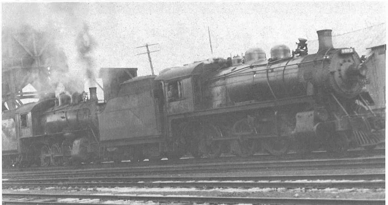
D10k 4-6-0 No. 1083 (built by MLW, October 1912, scrapped August 1960), and M4g 2-8-0 No. 3519 (built by Baldwin, June 1907, scrapped September 1959). Photo at Sutton P.Q., March 1932.
