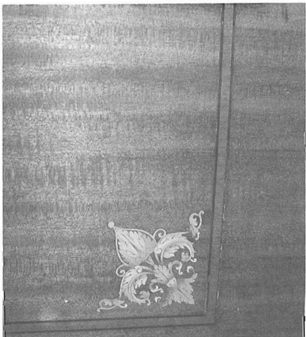
ABOVE LEFT: A corner of a section in car "Somerset" undergoing cleaning and repair to the mahogany veneer, on February 8, 1992, before varnishing. Note the delicate inlaid leaf motif in the upper berth.
