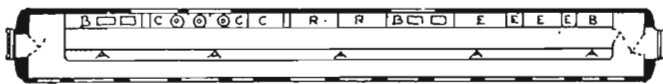
A - Service Counter (Bread & vegetable lockers, cutlery drawers, etc., below) B - Sinks C - Steamers R - Ranges E - Refrigerators
