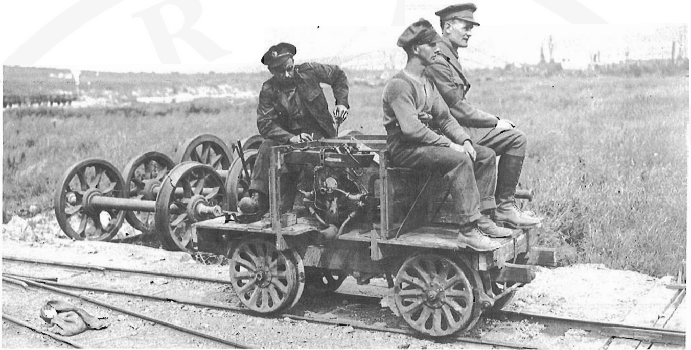
The "Mechanical Bug", a locomotive made by the Canadian Corps Tramway officers with the help of a corporal. The engine is from a motorcycle, the fly-wheel from a sugar refinery, and the belt from a minehead smashed by artillery fire.
