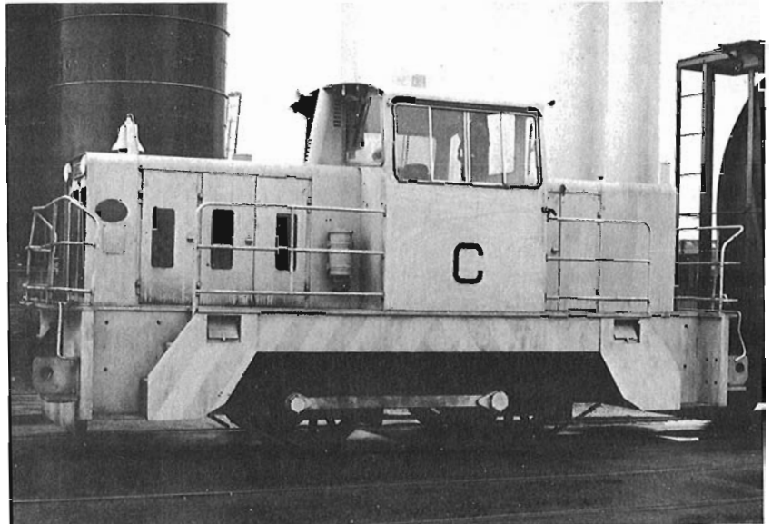
The third of the three Hunslet-built standard-gauge diesel-hydraulic 4-wheel switchers owned by Pacific Elevators Ltd. is seen going about its daily chores along the waterfront of Vancouver, B.C. in 1986, as it was then painted (Ronald Keillor)
