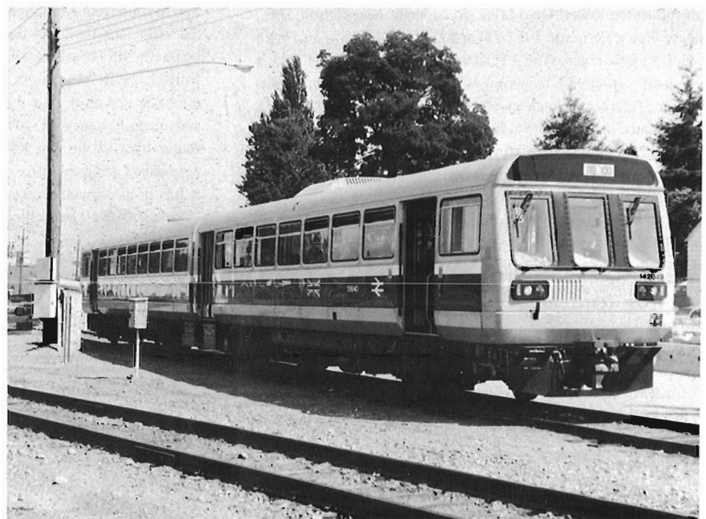
Two views of the BREL 2-car standard-gauge railbus #142049, on display at Abbotsford, B.C. (July 30, 1986) The upper view clearly shows the two-piece automatic folding doors. The temporary Railbus System connected with the SkyTrain, and passengers changed from one to the other at New Westminster, B.C. The SkyTrain service between Vancouver and New Westminster opened for public service in December 1985, six months before Expo started. (Both photos by Ronald Keillor)
