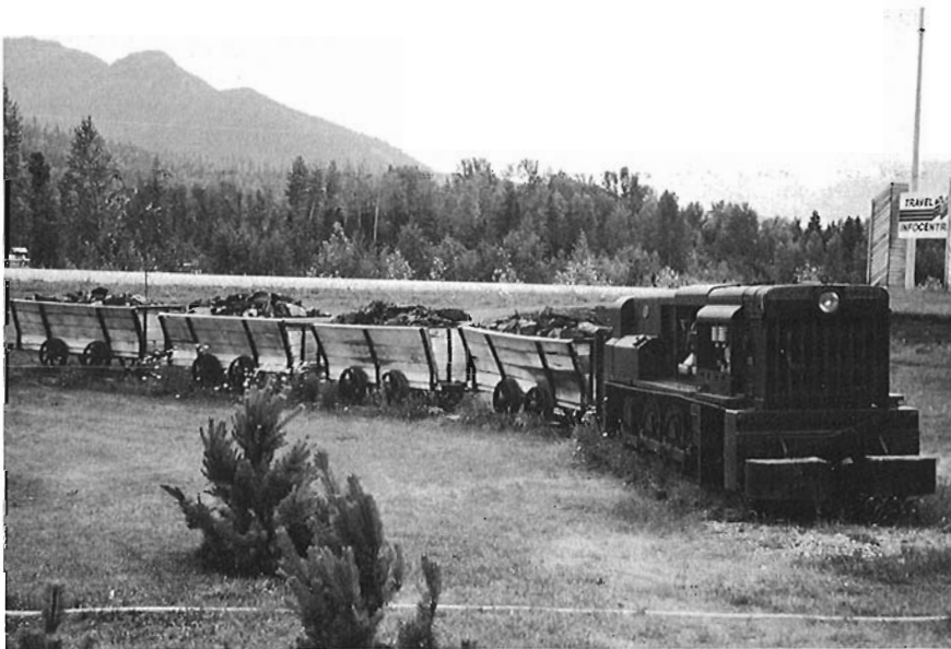
This 6-wheel Huwood Hudswell 36" gauge diesel mine loco is now displayed (1992) at the Fernie East, B.C. Infocentre with a 'train' of four 4-wheel wood-sided coal cars. (Lorne Nicklason)
