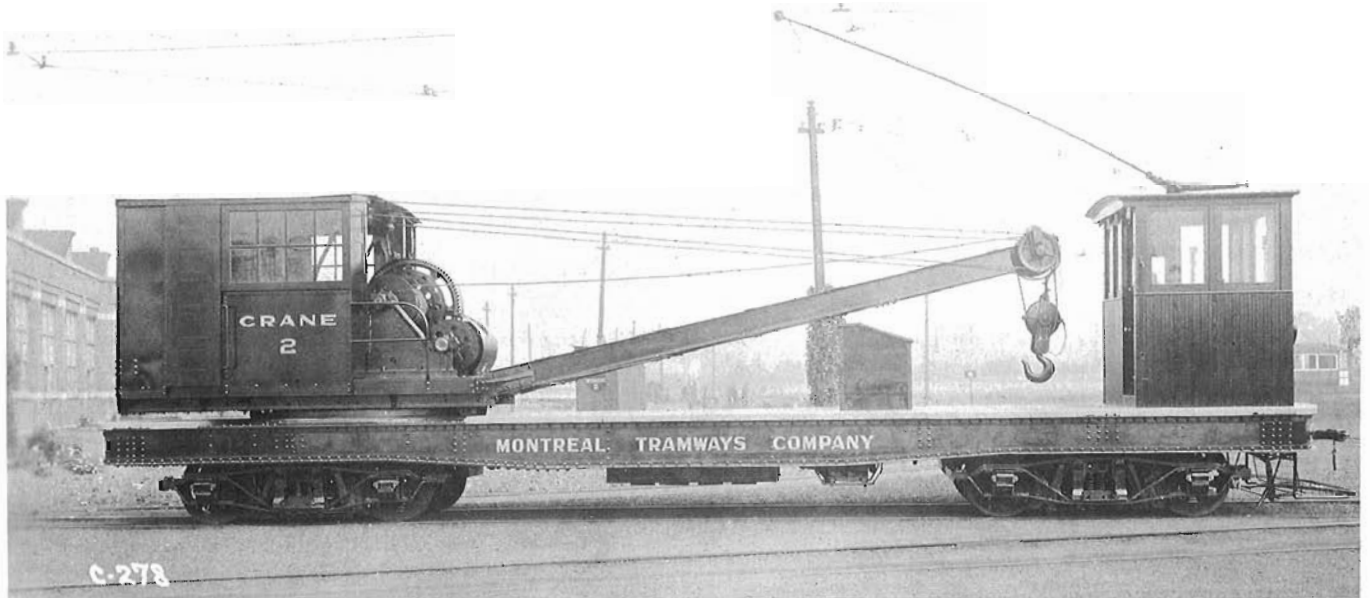
Montreal Tramways crane car No. 2, now W-2, as it appeared just after it was completed in the company's Youville shops in 1923. CRHA Archives, MUCTC collection.
