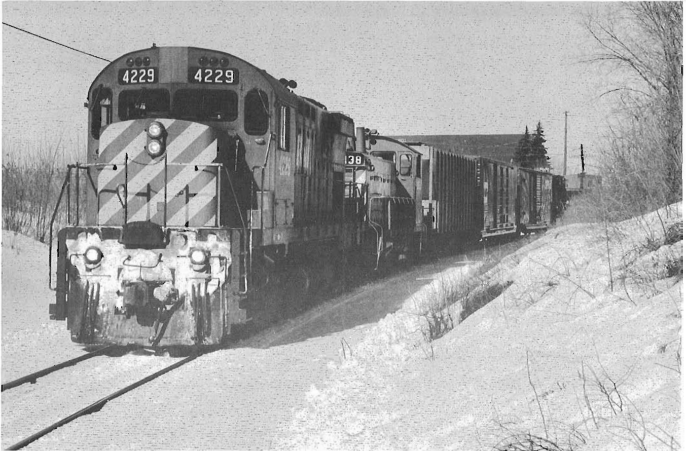
CP Rail Train 85 at Wamo Junction, Hull, Que., westbound to Walkley Yard on March 6, 1990. Motive power is C424 No. 4229 and SW1200RS No. 8139.
