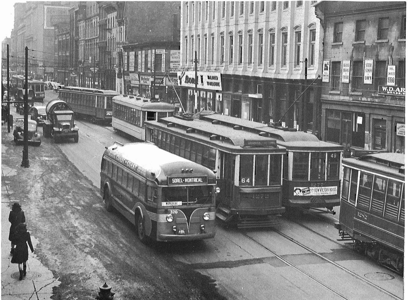
This photo, taken at the corner of Craig and Bleury in Montreal late in 1941, gives a good view of wartime operation of street cars. Ten trams are visible, many of them being the old "Montreal roof" 1200 class of 1911 to 1913. Note the sign on the back of 1277 saying "Come on Canada, buy the new Victory Bonds". The only bus visible is a long distance one from Sorel. CRHA Archives, Binns collection.
