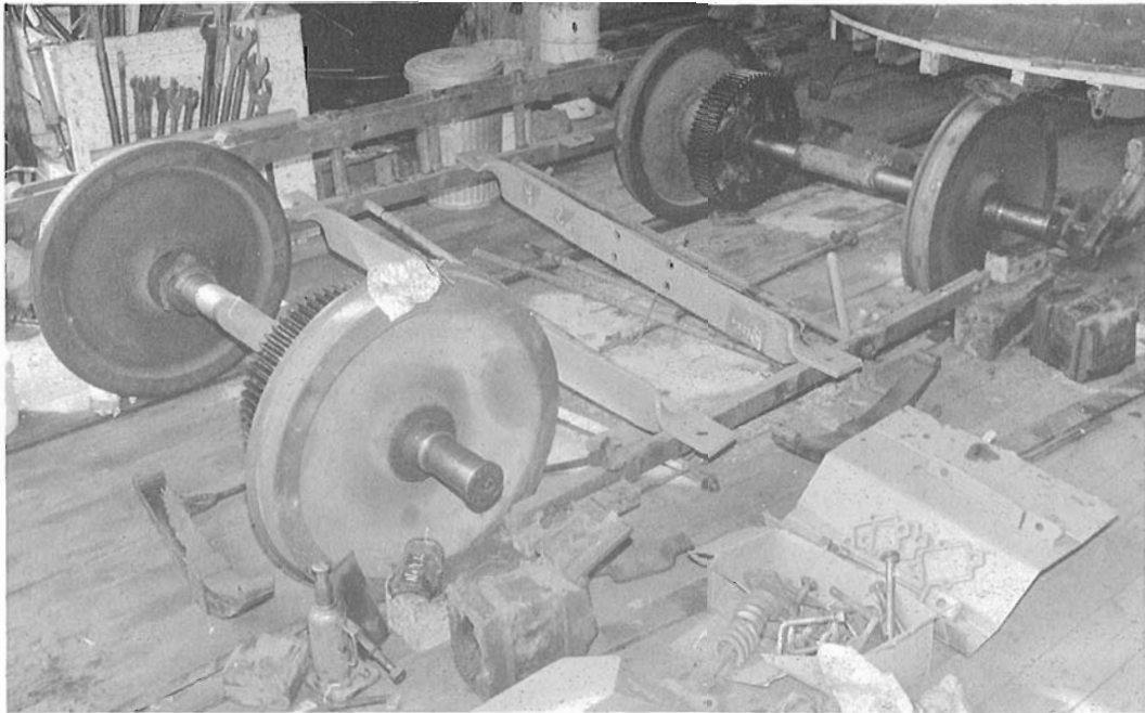
ABOVE: The truck of 15702 / 24 is almost completely dismantled in this view at the car barn on May 18, 1991. One side frame is to be replaced by a new one constructed in the shops. High Iron Photos 356-131-6b.
