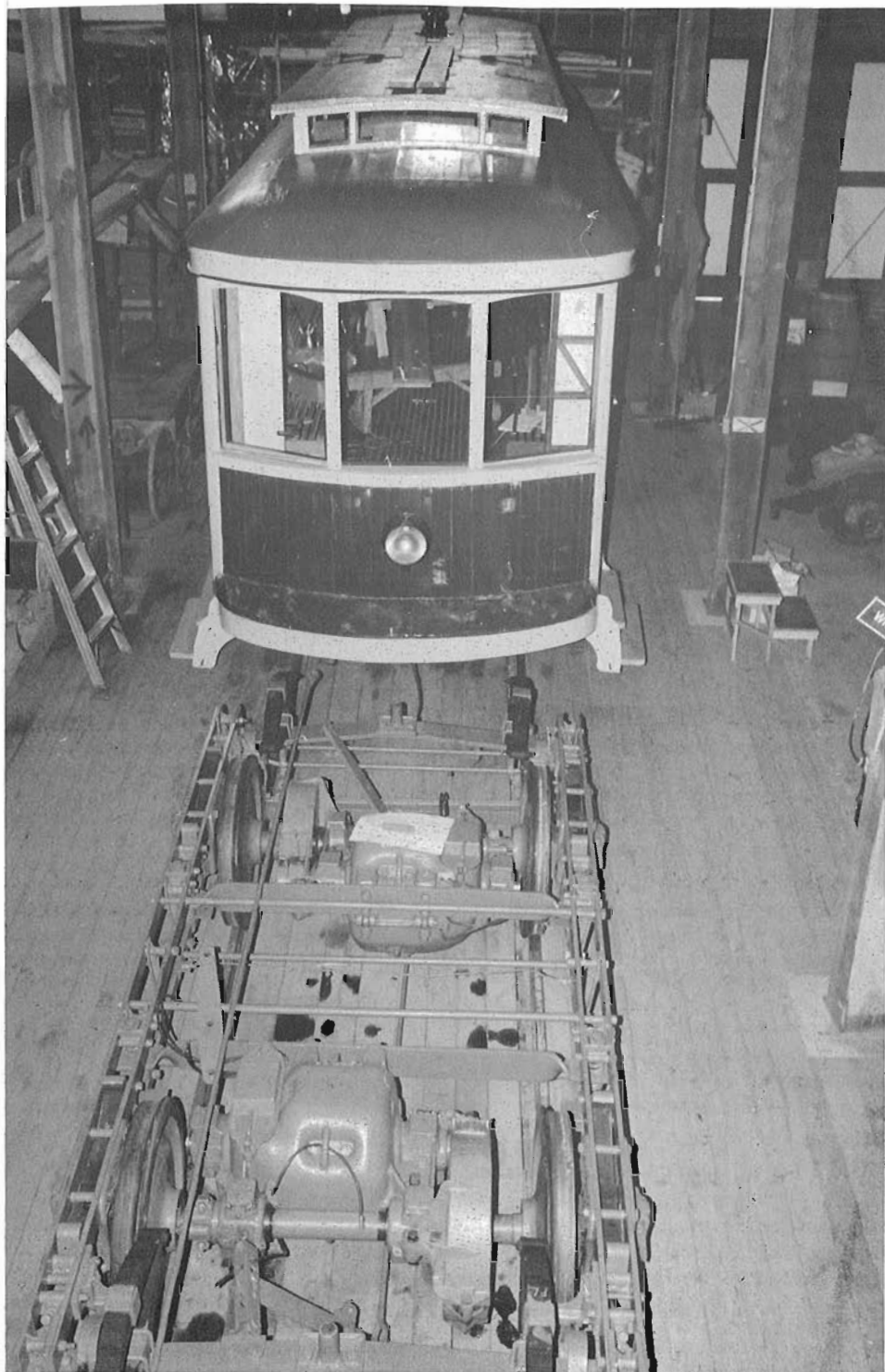
The rebuilt truck of ex-CNR 15702, (ex-Toronto Suburban Railway 24) ready to be run under the body on August 24, 1991. Note the GE 1000 traction motors, almost 100 years old and still fully functional. High Iron Photos 356-135-3a.
