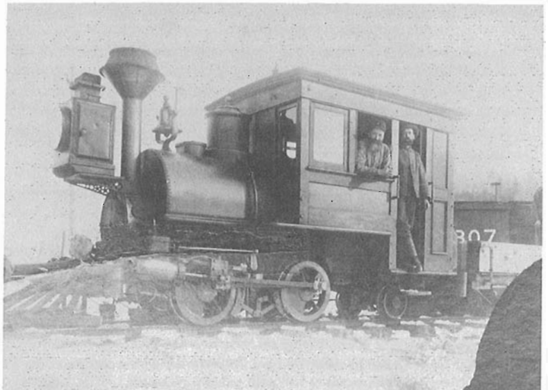
RIGHT: A small 0-4-2 locomotive of the New Rockland Slate Quarry near Kingsbury in 1894. This engine hauled slate from the quarry to Corris siding on the Grand Trunk Railway between Windsor Mills and Richmond. In the cab are engineer John McLean with his brother Archie McLean.
