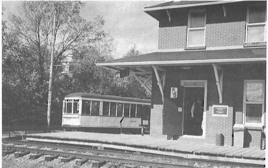
Ready to pick up passengers, MTC street car 1959 waits by the Hays building. Notice that the car is facing the opposite way than it did last year. This is to equalize the wear on the flanges as the car goes around the loop line.
