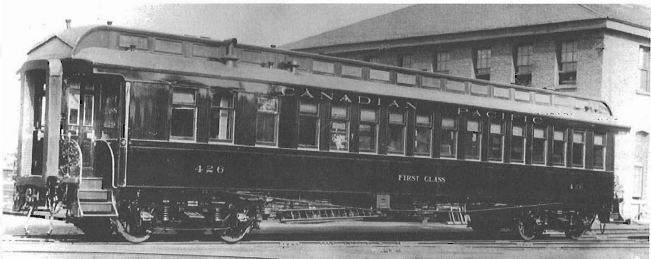
First class coach 426 was built for the Short Line service in 1890. It is much like 431 which derailed in the Palmer's Pond wreck, and in which Miss Patriquin was killed. Note the ornate narrow vestibules which were typical of the 1890s. Leach Collection.
