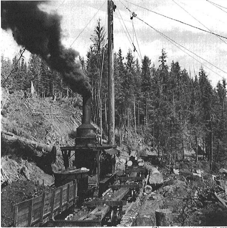
A typical landing scene from Allison's operations in 1940 shows a coal-fired donkey engine and spar tree used for yarding and loading the logs onto the logcars. -H. W. Weatherby photo, B.C. Forest Service, 2483-6
