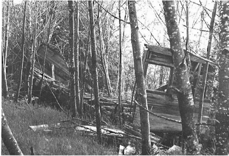
The body from a crew car remained at Aero Camp along with other equipment in 1971. This is probably the car shown in the photo of Shay No. 6. It was built either on the frame of a flatcar or from an old boxcar. -Robert D. Turner
