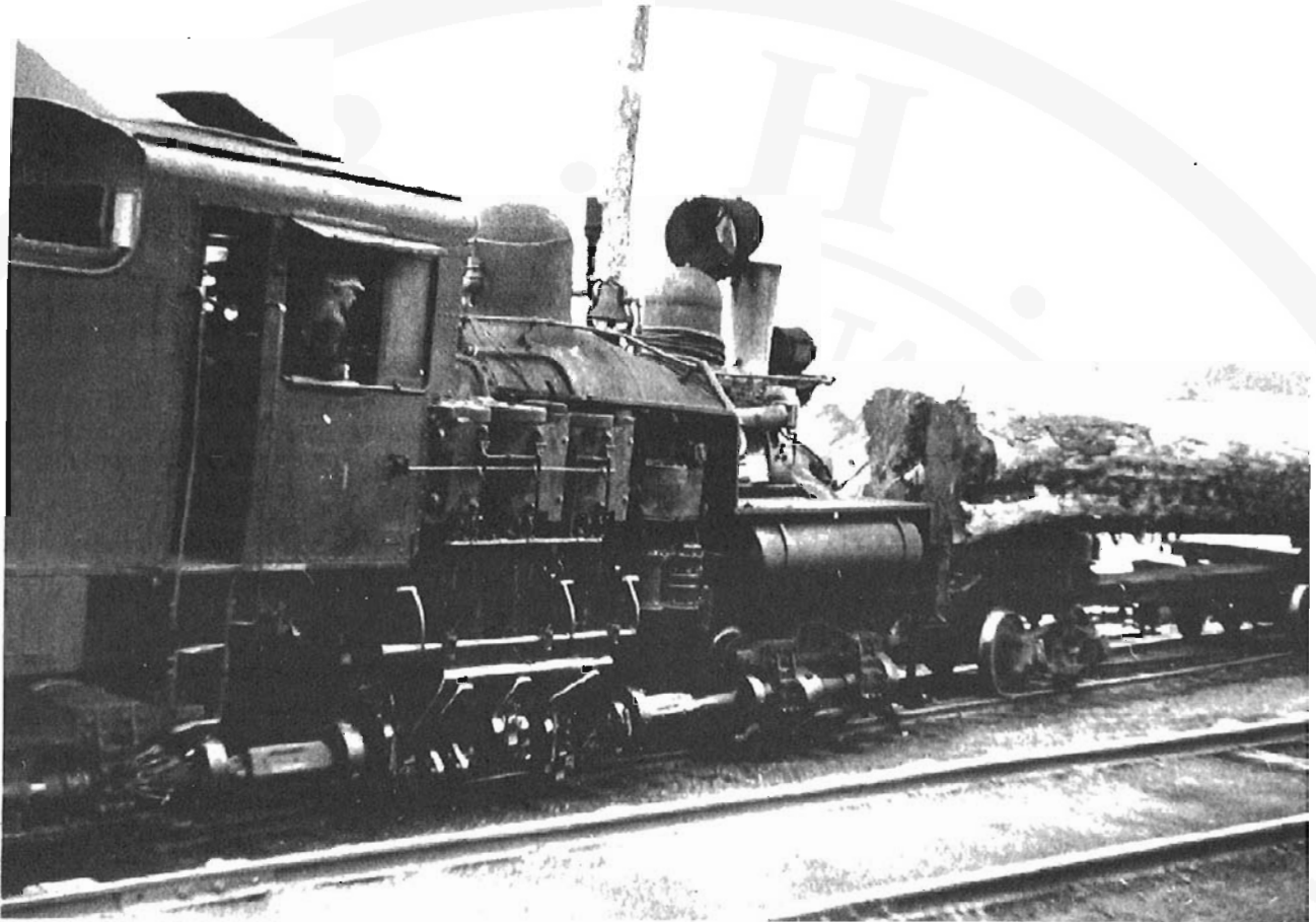
On the last log hauling day, August 31, 1955, Pacific Coast Shay No. 1 was in use. The generally rainy conditions on Morseby Island often made the use of the spark arrestor on the locomotive unnecessary. -MacMillan Bloedel Collection
