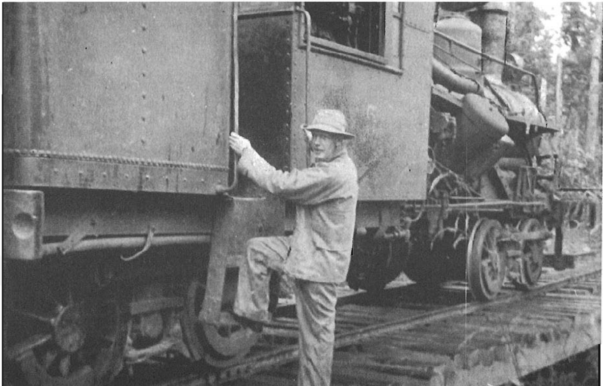
The three-truck Heisler became No. 5 for Aero Timber Company and often was used on the mainline between Skidegate Lake and the log dump. -MacMillan Bloedel Collection
