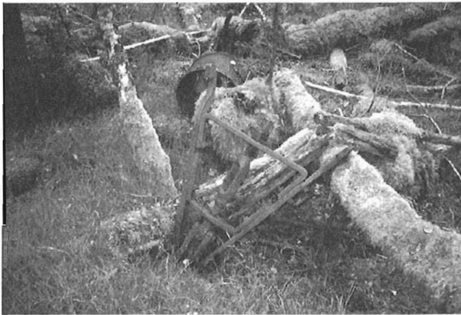
A manually-operated rail bender slowly rusts away. This is like the one used for many years by the volunteers at the Canadian Railway Museum.
