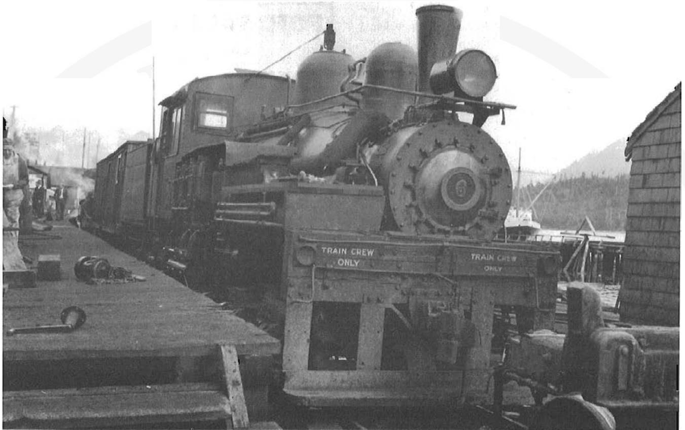
Three-truck Shay No.6 with a crew car at Aero Camp. The Union Steam Ship Company's Coquitlam (II) is in the background. -Maurice Chandler Collection
