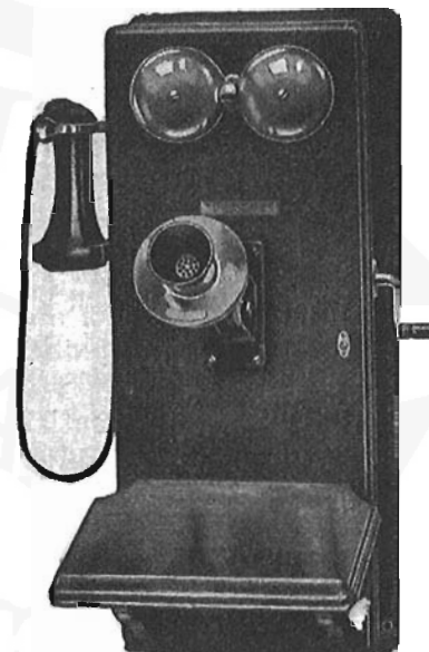
ABOVE: This is the type of telephone that was used to spread the news. To make a call, you turn the crank which operates a magneto generator. This signals the operator, or the other phones on the party line. Then you take the receiver off the hook and listen for the answer. Telephones like this were still in use in some rural areas well into the 1950s.
