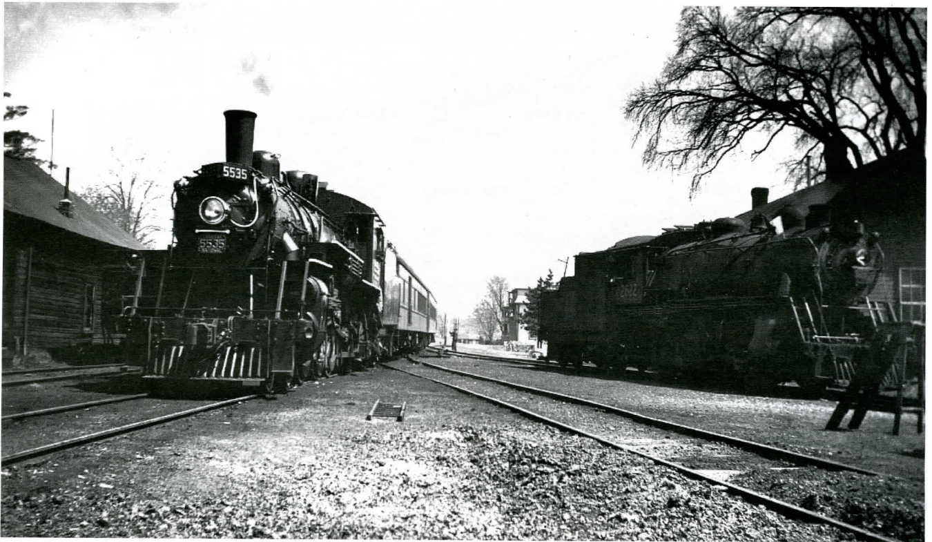
The local freight engine, 2622, a 2-8-0 Consolidation, was built in 1911 for the Grand Trunk and was scrapped in 1958.
