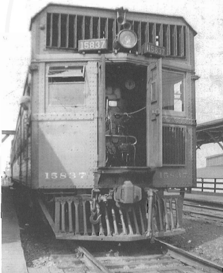
A view into the engine room of 15837. The engineer sat right beside the diesel engine, but on a hot day enjoyed the breeze through the open front doors. Photo by Lorne C. Perry
