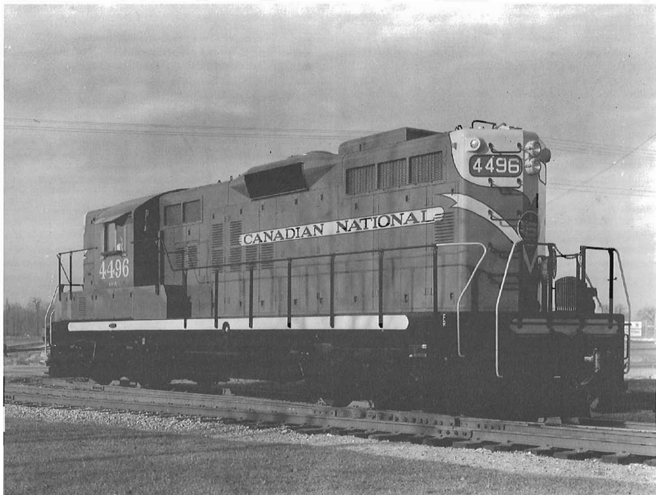
CN 4496 ably demonstrates the distinctive profile of a General Motors "Geep", in this case a GP9. Note the dynamic brakes. CN photo 52683-1.
