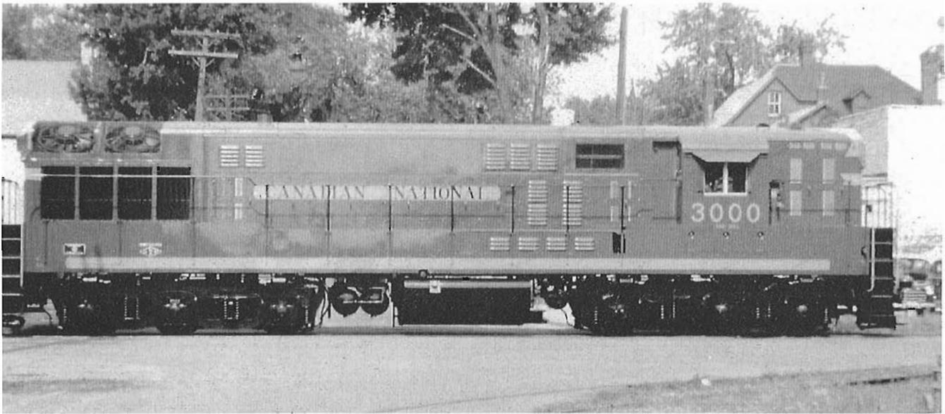
*Trainmaster in profile - 2,400 horsepower in one unit.*
