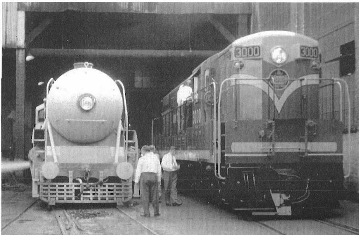
*The two eras side by side. An Indian State Railways Pacific type is exhausting steam following a boiler test, standing on its broad gauge track, while CNR's new Trainmaster is carefully inspected.*
