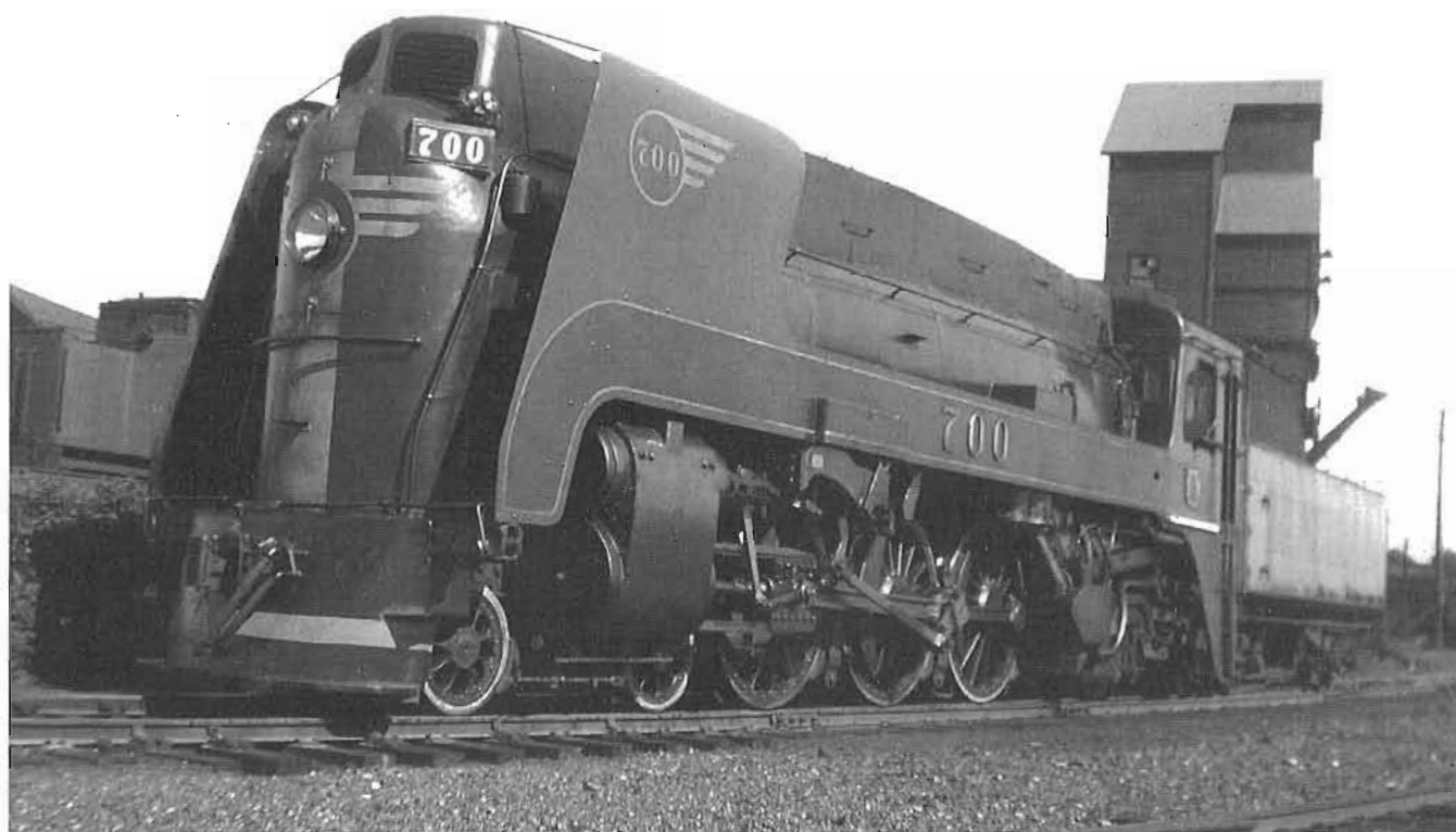
No. 9. Temiskaming & Northern Ontario 700, 4-6-2 Pacific. North Bay, Ontario, 12 September 1943 Collection : Hugues W. Bonin (bought from Dave Shaw)
