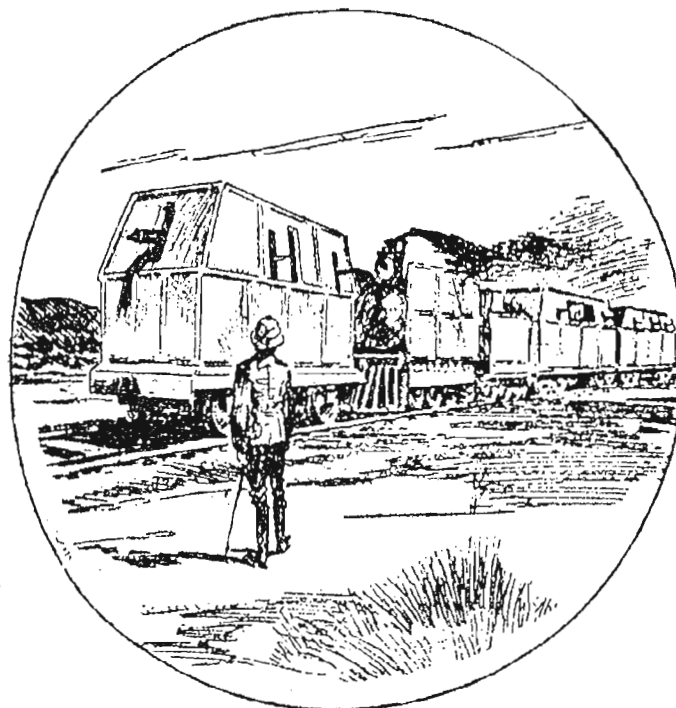
TOP: A drawing of an armoured train out on patrol in South Africa in 1899. The protection here is less than on some other trains. Collection of Weldon McLean.
