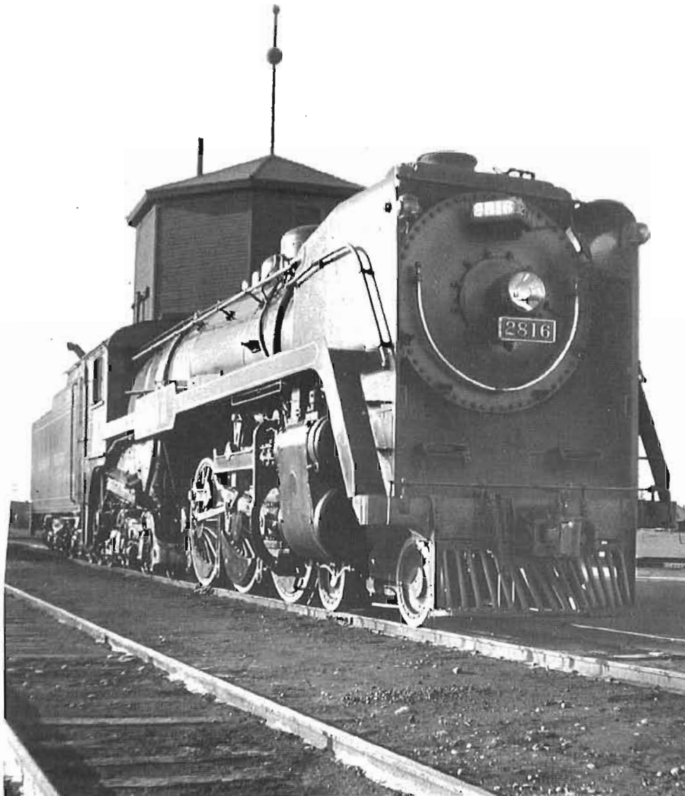
No. 7. Canadian Pacific 2816, 4-6-4 Hudson. Calgary, Alberta, (No date) Collection : Hugues W. Bonin (bought from Dave Shaw)
