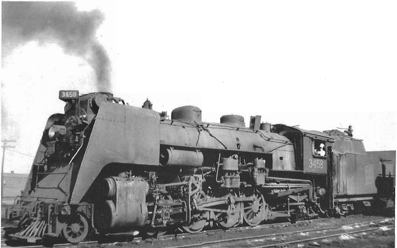
No. 4. Canadian National 3458, 2-8-2 Mikado. Ottawa, Ontario, July 1947 Collection : Hugues W. Bonin (bought from Dave Shaw)
