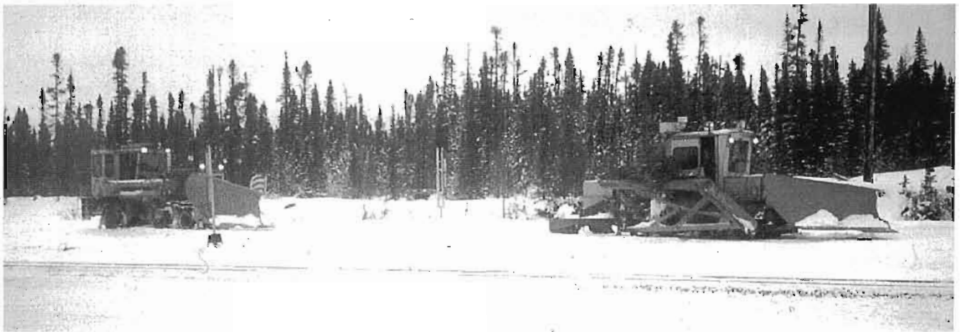
ABOVE: The modern way of clearing snow from tracks is exemplified by these ploughs, which can run on track or road. They are seen at Ross Bay Junction on the Quebec North Shore and Labrador Railway on December 16, 1999. Photo by Fred Angus
