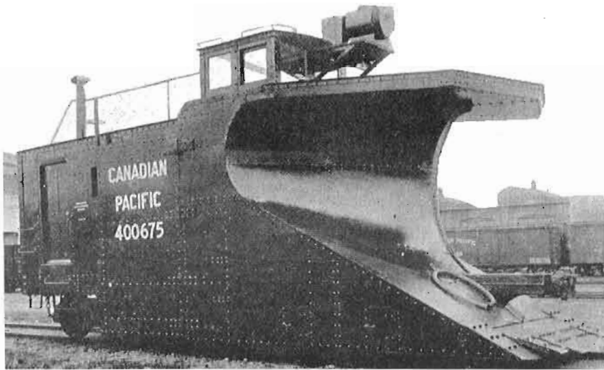
Fig. 12. Single track, steel snow plough, Canadian Pacific Railway.
