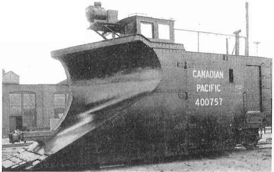
Fig.13. Single track, steel snow plough, Canadian Pacific Railway.
