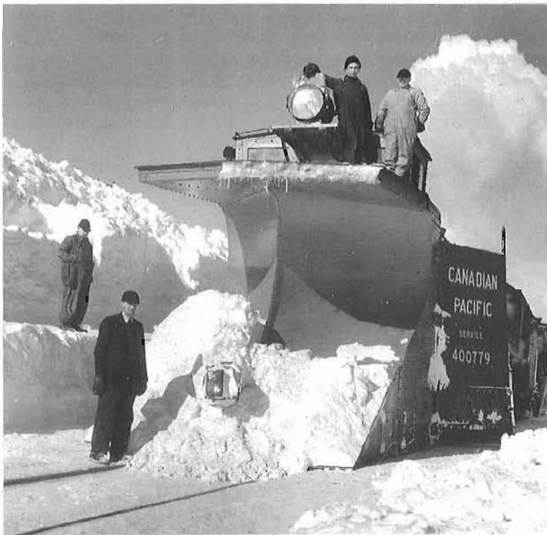
ABOVE: This snow melter was photographed in action in February, 1948. It was useful in yards where there was little room to dump the snow. Canadian Pacific photo No. 12418.
