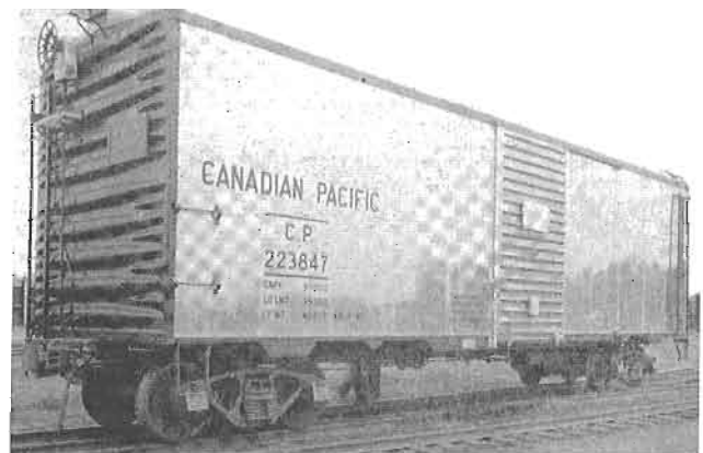
The CPR ordered aluminum box cars to save steel and reduce weight.
