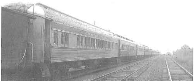
1968 saw the end of one of the most interesting series of passenger cars in Canada, CP's "U" class tourist cars. They were old heavyweight cars sheathed with stainless steel for use on "The Canadian". Retired in 1966, when the "Dominion" was taken off, some were placed in storage. This photo was taken at Delson on June 22 1968 when the last of the group was on the way to Farnham for scrapping.
