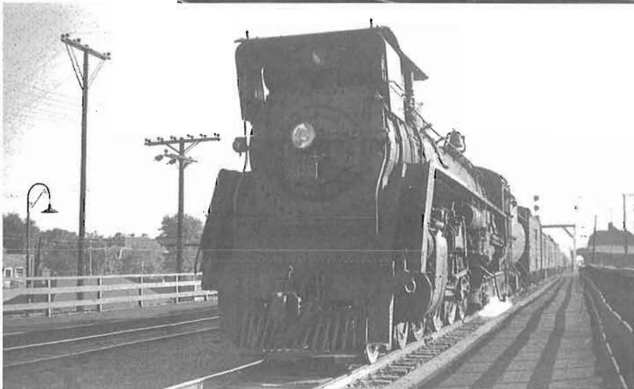
ABOVE: 6176 with an experimental smoke deflector, as seen at Truro Nova Scotia in 1951. Collection of Dave Shaw
