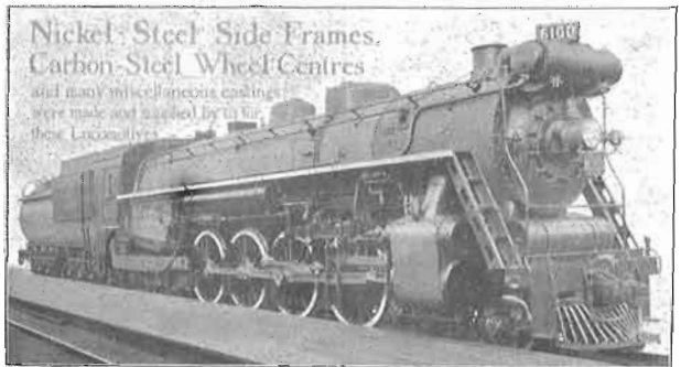
4-8-4 "Northern" Locomotive for Canadian National Railways. Built by Canadian Locomotive Company, Limited.
