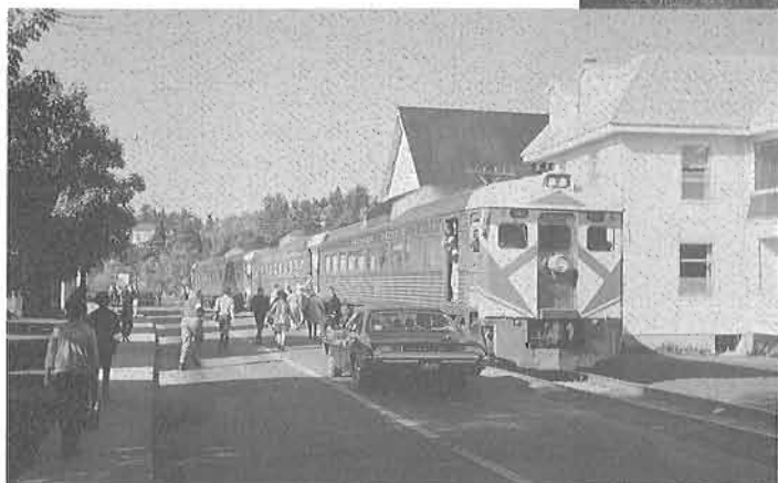
RIGHT: Oldest of the CPR's Budd car fleet was 9116 which was built in 1951 as Lehigh Valley No. 41. It was remembered by commuters for its low-back seats. In this photo it heads a three-car commuter train on December 6, 1969.
