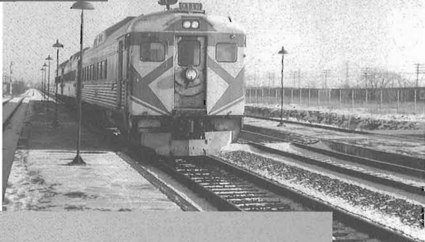
RIGHT: Oldest of the CPR's Budd car fleet was 9116 which was built in 1951 as Lehigh Valley No. 41. It was remembered by commuters for its low-back seats. In this photo it heads a three-car commuter train on December 6, 1969.
