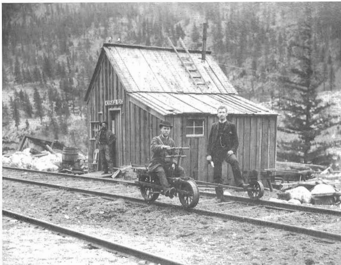
A very early photo of a velocipede in B.C. taken about 1890 on the CPR main line at Cisco where the track crosses from one side of the river to the other in the Fraser Canyon, 150 rail miles east of Vancouver. Vancouver Public Library Special Collections, No. 232
