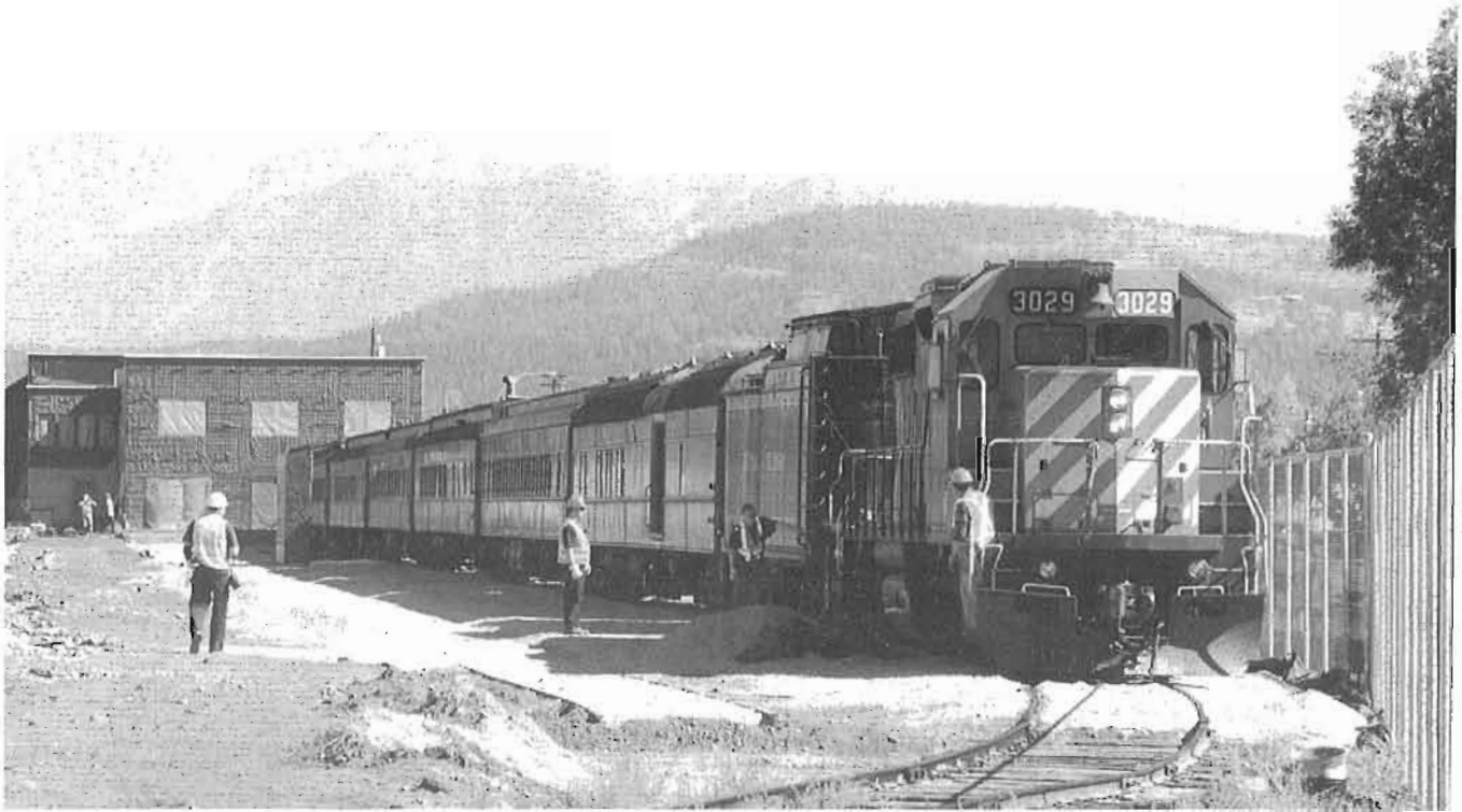
GP38-2 No. 3029 spots the Trans Canada Limited up to the end stops on Track 1.
