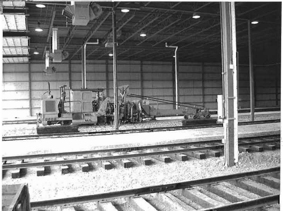
RIGHT / DROIT: Coyle's tamping and levelling machine at work in the great hall. (GH)
