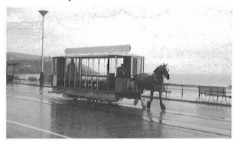
Car No. 49 is one of three convertible cars built in 1935, the newest cars in the Douglas horsecar fleet. They are open cars which can be converted to closed in bad weather.
