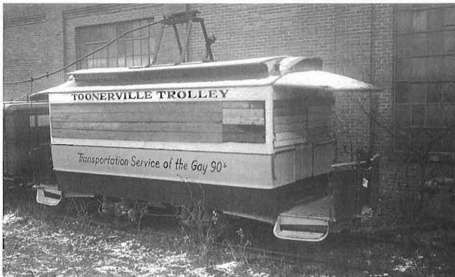
**This strange vehicle is obviously a horsecar converted to electric operation, while still retaining its pedestals. Amazingly it was photographed as recently as November 21 1943 in Kitchener Ontario. It was probably a passenger car of the Berlin & Waterloo Street Railway, later used as a work car. Its final disposition is unknown.**
