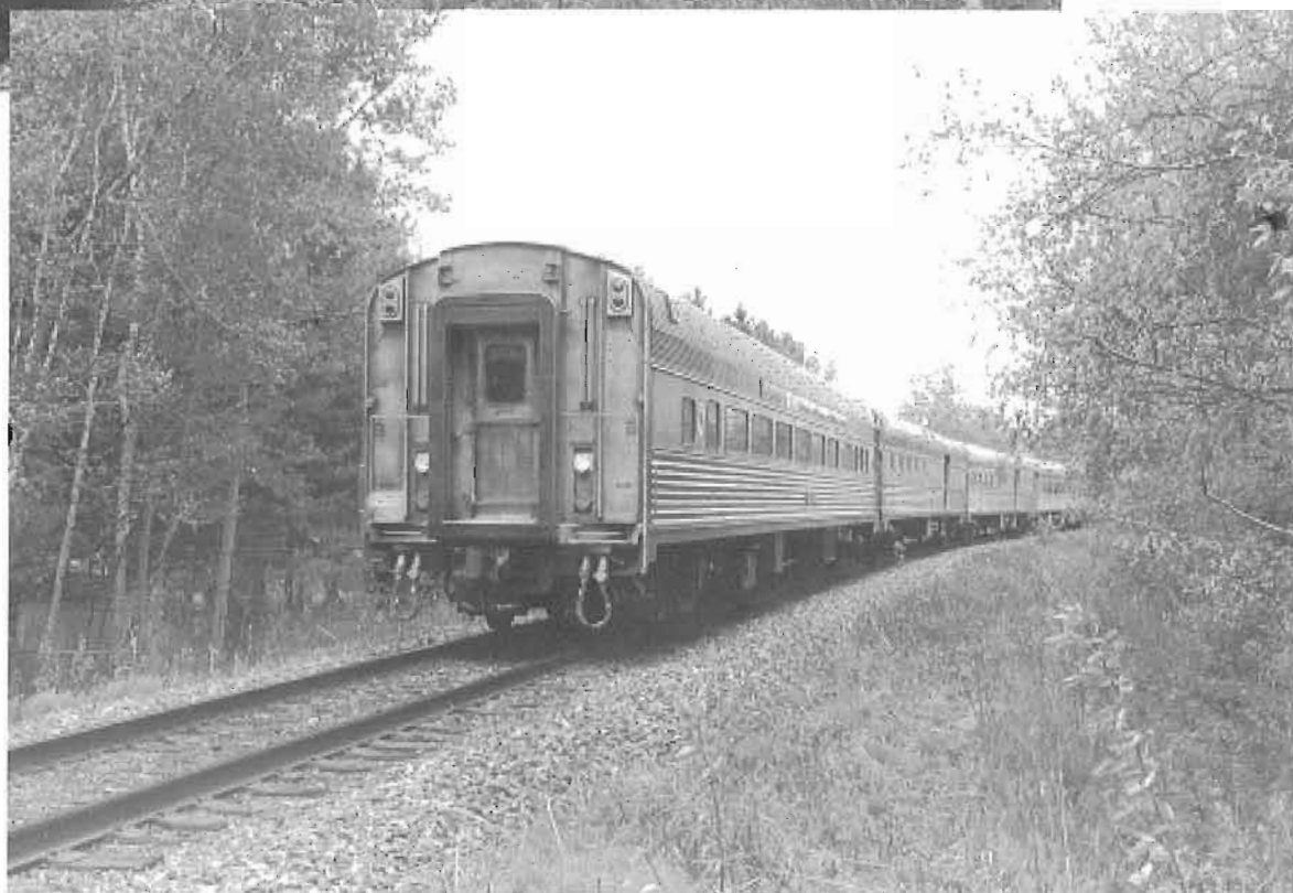
Opposite and above we see three views of No.601-603 climbing the stiff grade between Grand'Mere, 111 miles out, and Garneau, a division yard, 115 miles out on Friday, 23 May 2003. The two baggage cars, numbers not recorded, are ex-Canadian Pacific Budd stainless steel cars. The coaches, numbers not recorded either, were bought from various sources in the U.S.A. and thoroughly rebuilt. Compared to the larger windows Canadians are accustomed to, the "slit windows" of these coaches were a first experience for your photographer. The train splits at Hervey, 19 miles beyond Garneau: one section proceeds northeast and north to Jonquiere, Quebec; the other turns northwest and west to Senneterre, Quebec. All photos by Gordon D. Jomini
