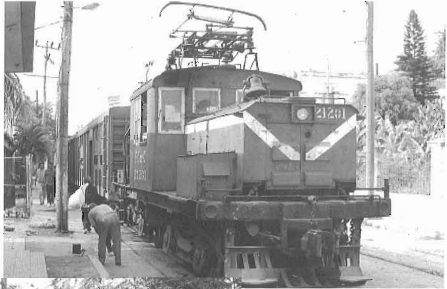
RIGHT AND BELOW: Train, hauled by a 1200 volt box cab electric locomotive, loading at Havana. Note the box cars converted to passenger cars.
