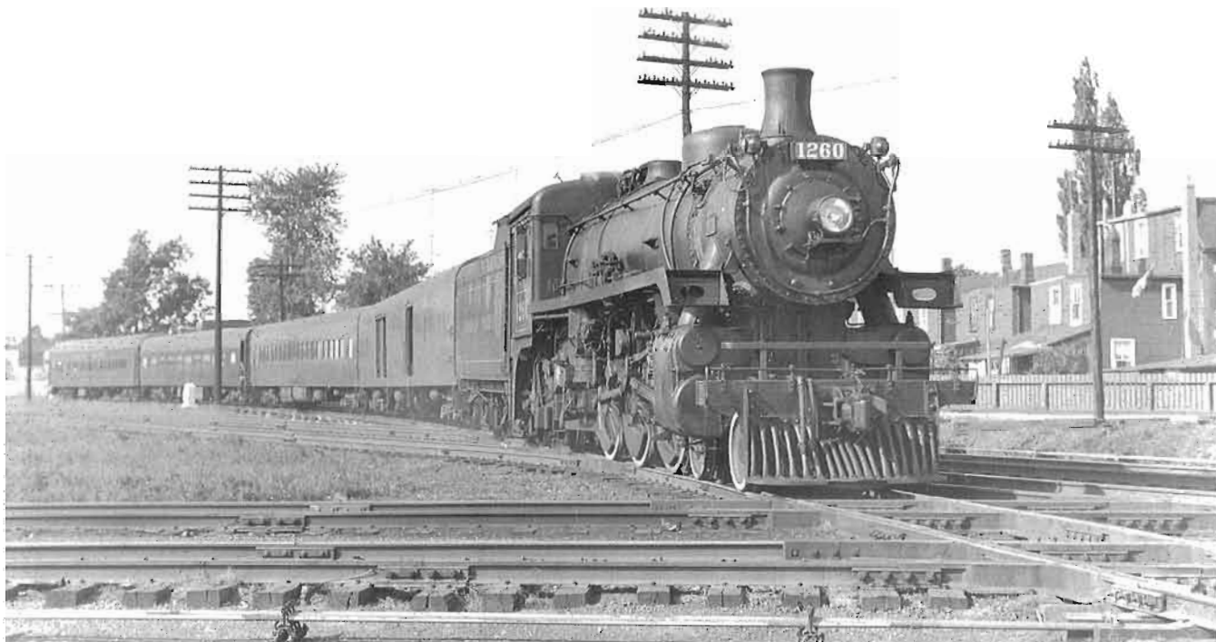
CP No. 26, an all-stops local train from Sudbury, is seen clattering across the West Toronto diamonds in this 1955 view. G5c Pacific No. 1260 was only nine years old when this photo was taken, and it would be scrapped in 1961. Photo by Al Paterson
