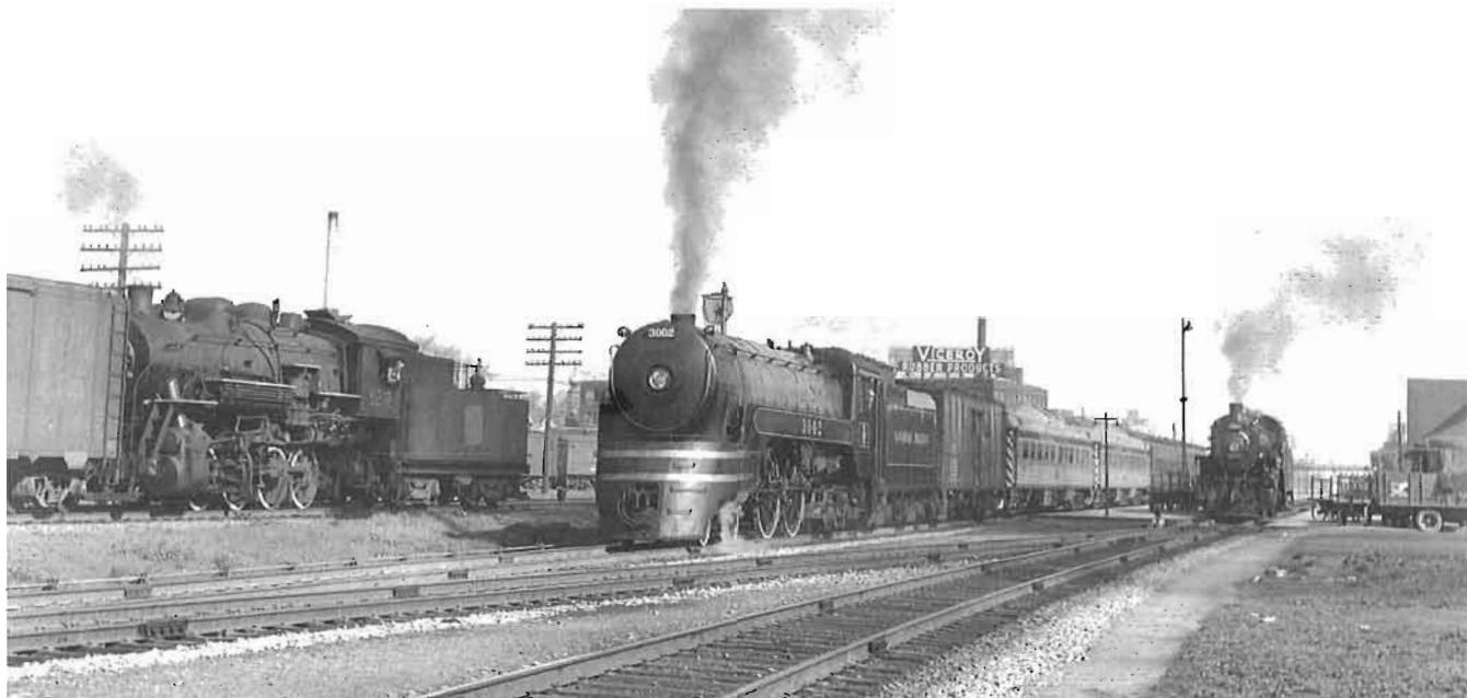
CP No. 629, westbound for London, pauses at West Toronto in May 1954. The previous year, Rail Diesel Cars had taken over this run, but heavy weekend traffic required extra coaches and a locomotive. Engine No. 3002 is a streamlined 4-4-4 Jubilee, built by the Montreal Locomotive Works in 1936. On the left CN No. 8202 is running in reverse with some freight cars, while CP No. 3727 simmers in front of the station waiting for the passenger train to clear the crossing. Photo by Al Paterson
