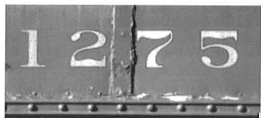
BELOW: A closeup of the number on the side of 1275 showing the removable side panels intended to make it easier to repair dents such as the car shows in the photo above.
