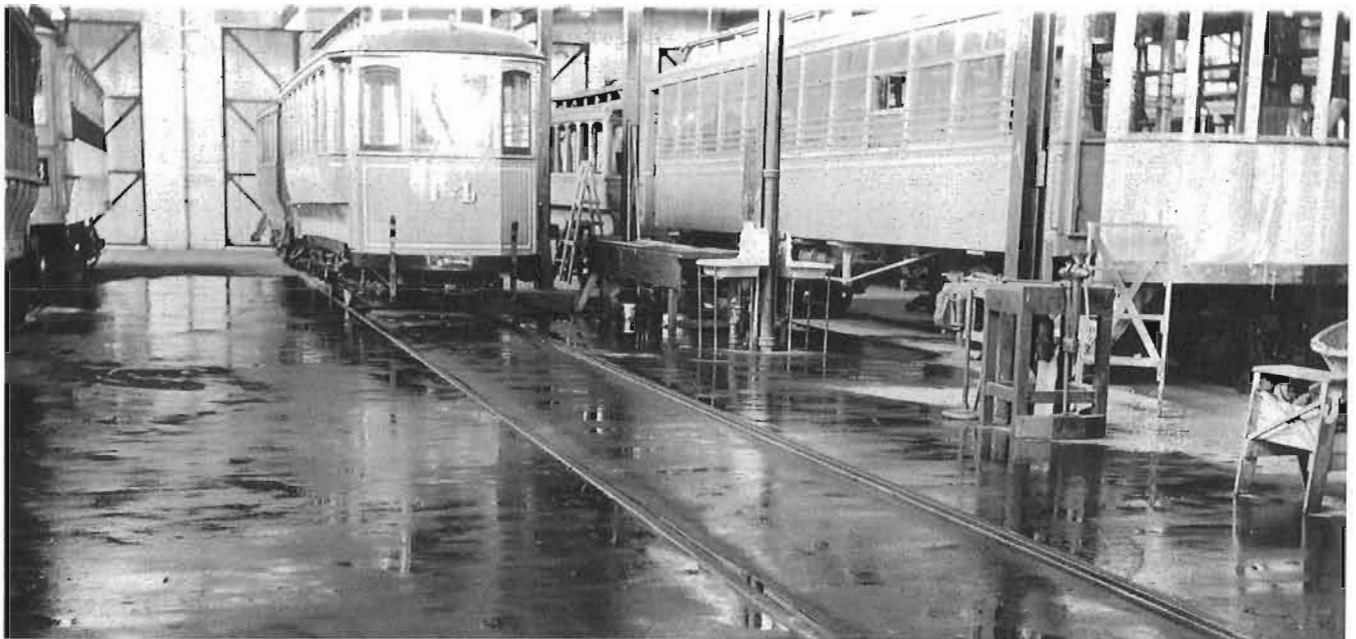
An assortment of no less than six cars, all different, in Youville Shop in 1912. From left to right we see: A single-truck open car built in 1899, A suburban car of the 1031 class, formerly open but converted to closed, A former open car rebuilt as a convertible in 1905, Former Montreal Terminal Railway closed car 14, An early closed electric car looking rather the worse for wear, A 1032 class former Park and Island suburban car.
