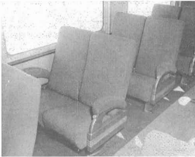
Seats in new C.N.R. first-class coach. The seats, except at the bulkheads, are reclining and rotating, with foot rests. The view at the right shows the seating arrangement at the bulkheads, with removable lightweight table in position.
