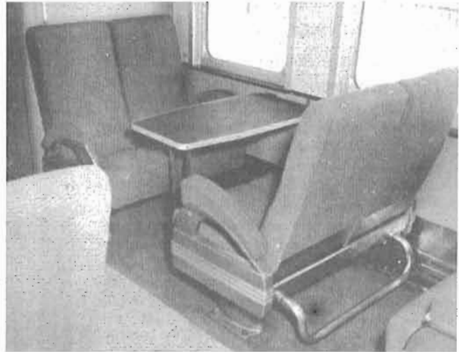
Seats in new C.N.R. first-class coach. The seats, except at the bulkheads, are reclining and rotating, with foot rests. The view at the right shows the seating arrangement at the bulkheads, with removable lightweight table in position.
