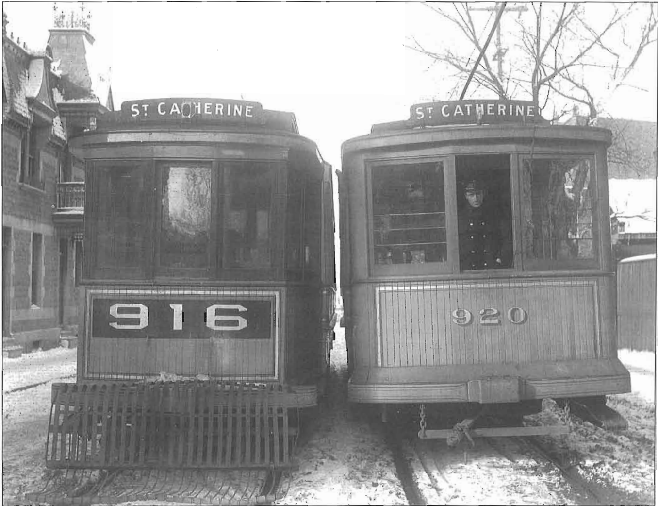
Two "first generation" PAYE cars (916 and 920) pass each other late in 1905 or early in 1906. The large red number plate on 916 is plainly visible, as is the Sleeman fender. There certainly is not much clearance between the two cars; it is time to re-align the track on which 920 stands, for the car has a pronounced lean. CRHA Archives, Fonds Montreal Tramway Company, P042.
