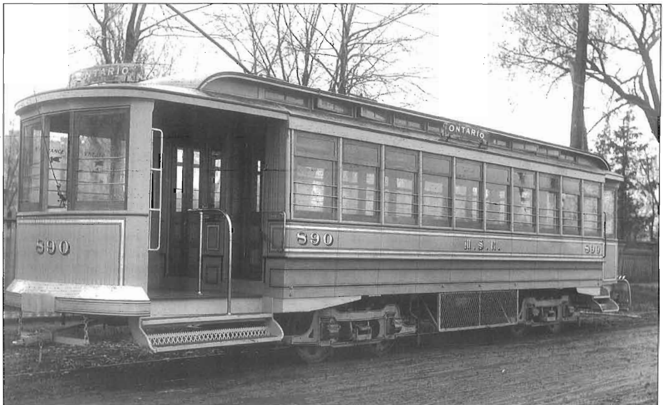
The World's first Pay-As-You-Enter car, No. 890 just after its completion early in May, 1905. The rear platform, brass rails and double doors are plainly visible. CRHA Archives, Fonds Montreal Tramway Company, P042.
