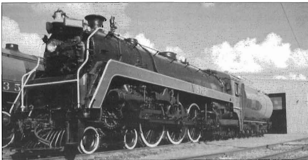
5702, one of two preserved 5700's stands proudly outside Exporail's building number 5 where it is on permanent display. 5702 had been hauled out and spotted for the 2004 'Iron Horse Weekend' at Exporail. It's 80 inch diameter driving wheels continue to amaze the children that are posed for photographing beside them! Photo, Stephen Cheasley.
