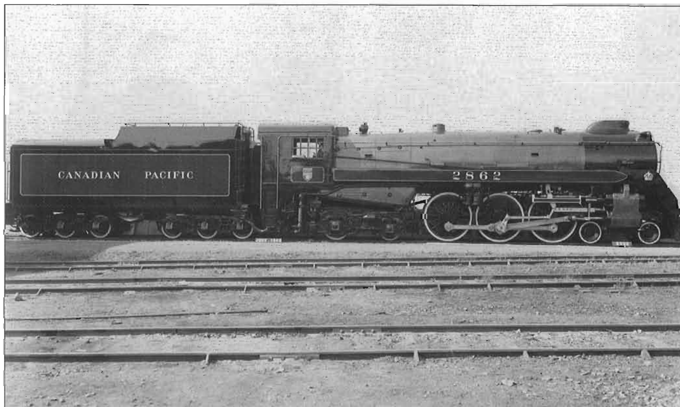
CPR Hudson class H1e, road numbers 2860 to 2864, 5 units built by Montreal Locomotive Works in 1940. 2862 was officially photographed at MLW prior to delivery in 1940. Photo CRHA Archives, Fonds Corley.
