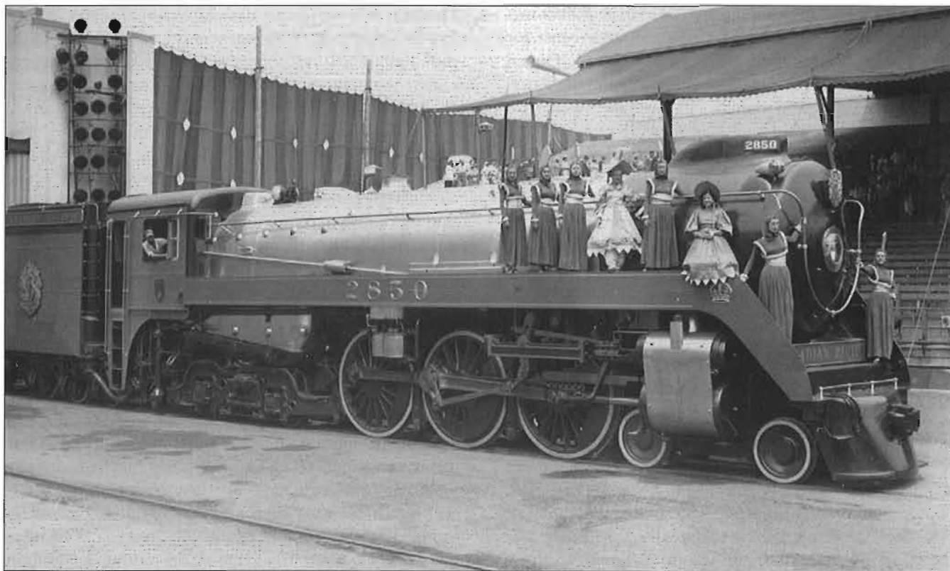
CPR Hudson class H1d, road numbers 2850 to 2859, 10 units built by Montreal Locomotive Works in 1938. After pulling the Royal train across Canada, 2850 was exhibited at the New York's World Fair in 1939. Photo CRHA Archives, Fonds Corley.
