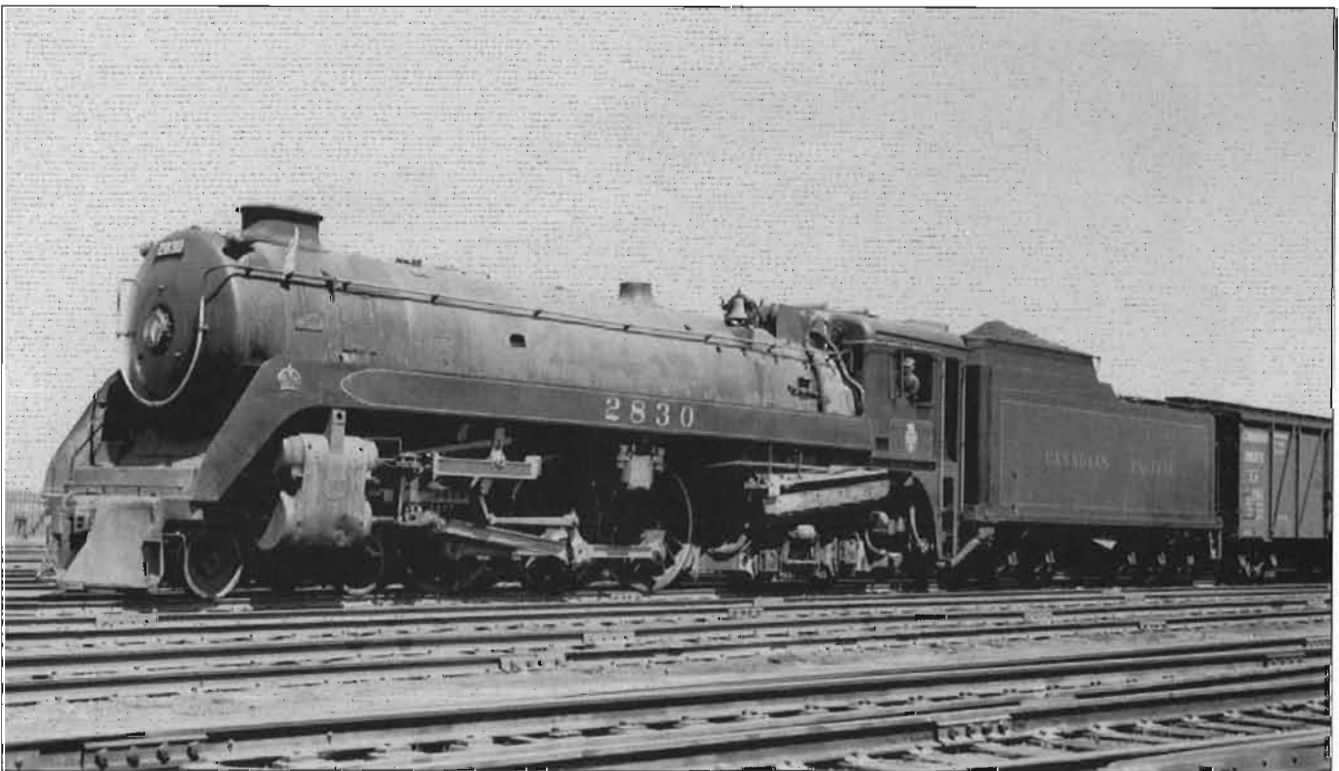
CPR Hudson class H1C, road numbers 2820 to 2849, 30 units built by Montreal Locomotive Works in 1937, these were the first Hudsons to be given the 'Bowen treatment'. 2830 was photographed hauling a freight at Winnipeg, Manitoba in July, 1948. Photo CRHA Archives, Fonds Corley.
