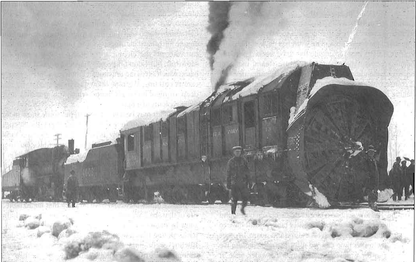
In mountainous regions, the big rotary ploughs were called into service. 400811 was the newest of ten rotaries on the CPR roster in 1938. Photo, Canadian Pacific
