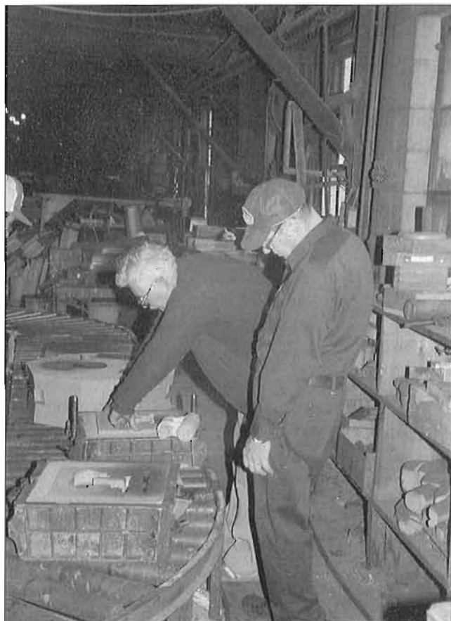
Readying the moulds at the foundry, preparatory to casting the cylinders for locomotive 5606. Photo Ed Farley
