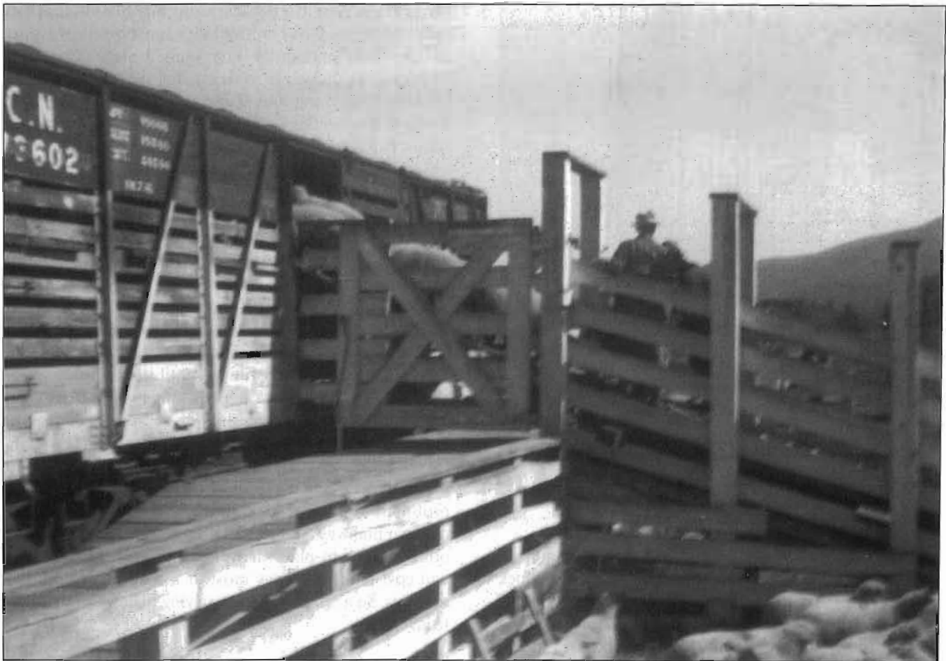
Loading sheep photo. Loading sheep at Birch Island in 1962 onto top deck of CN stockcar No 173602. It is believed to be a relatively 'modern' car, having being rebuilt from a 1913 boxcar in 1949-50. It had 6 ft. wide doors. Moilliet family.
