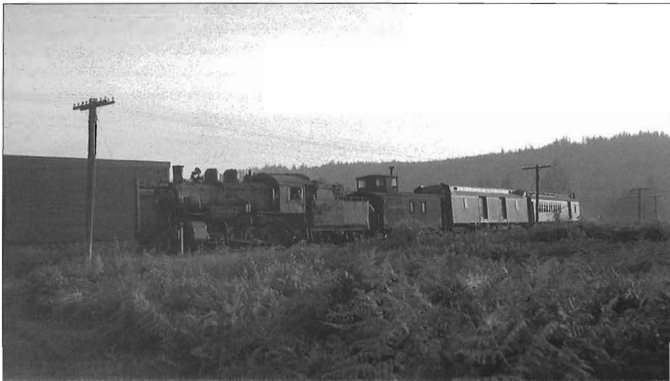
Running northward on the Westminister Branch, CP class M4f Consolidation locomotive 3458 nears Coquitlam station with a caboosé, a mail and express car, and a passenger/baggage combination car, on August 24, 1942. The line saw few passengers, and the conductor and two brakemen rode in the caboosé. (Addison Lake collection)
