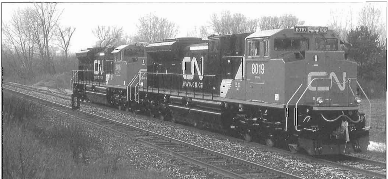
CN SD70M2s 8019 and 8016 on the running test track at Electro-Motive Canada Ltd. in London, Ontario on January 6, 2006. The two units were delivered to CN on January 10, 2006. The units were delivered in two lots: CN 8000–8019 in 2005 and 8020–8024 in 2006. Photo by Gordon R. Taylor, Don McQueen Collection.
