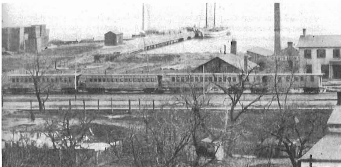
Grand Trunk passenger cars in Toronto about 1856. The 14-window cars are likely built in Montreal by the English contractors, using iron hardware manufactured by the Canada Works in Birkenhead. The 15-window car, second from left, was probably built by a Canadian builder. Note that the English cars have spoked wheels.
