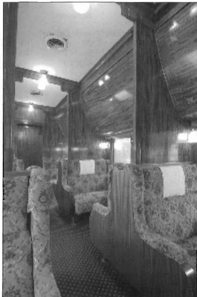
First class sleeping car 'Rutherglen' (1929 Trans Canada Limited set) showing inlaid quarter-sawn Honduran mahogany panels.
