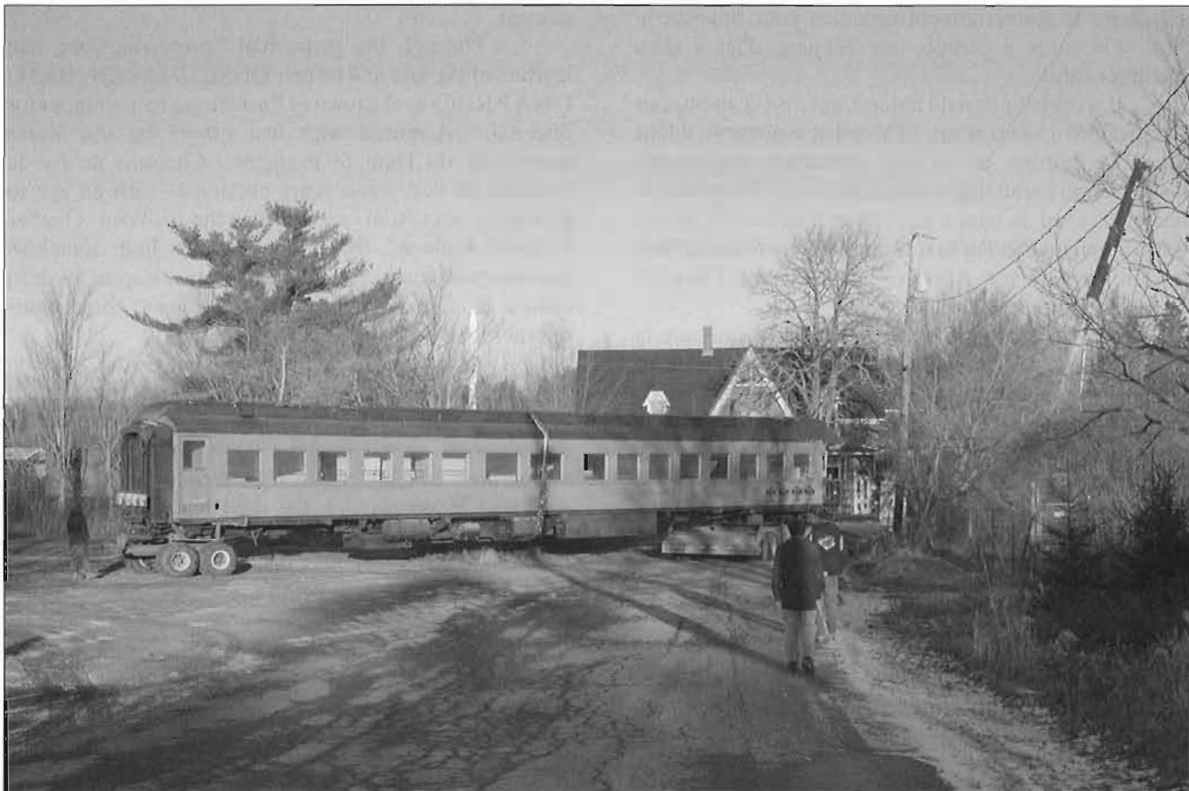
The "Alexandra" is arriving at its new home at the Train Station Inn in Tatamagouche, Nova Scotia at 1512 on Wednesday, December 20th, 2006. Phil Leil Enterprises Ltd. of Truro handled the move and prepared a specially fabricated, hydraulically-actuated dolly capable of making right angle turns in Amherst and Tatamagouche. Both photos courtesy Bill Linley.
