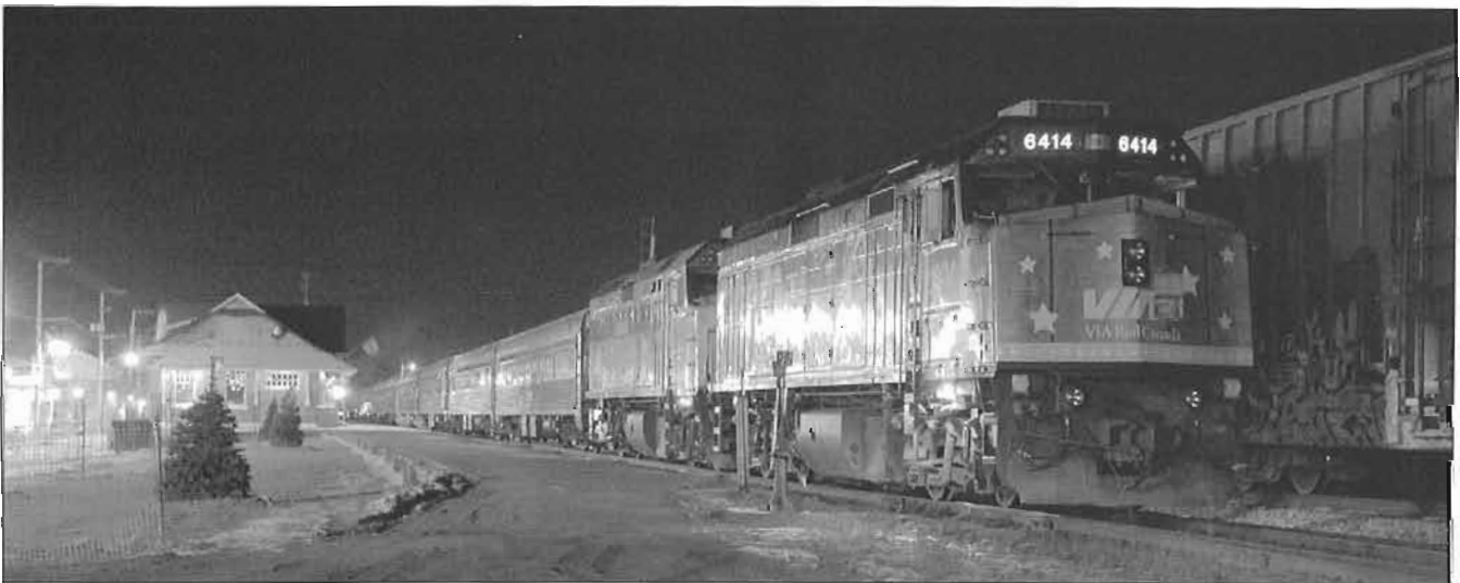
On Tuesday, November 21, 2006 VIA ran a test of a J-Train from Montreal to Matapedia to examine the feasibility of simplifying the switching necessary to cut the Chaleur in and out of the Ocean at Matapedia, Quebec. The Eastbound train consisted of a typical full-summer consist of the combined Chaleur and Ocean. The Chaleur had 8 cars with two units followed by a further two units and 18 cars of Renaissance Stock and a Park Car. Train 614 is seen at Mont Joli during a brief stop at 0449 on Wednesday, November 22nd. Only limited stops were made on the eastbound run to assess the braking characteristics of the train. The train continued on a non-stop run to Matapedia, turned on the wye and the four units were remarshalled to the head end for the return trip to Montreal. The consist included 6414 6424 4122 4105 4115 4100 4102 4104 4116 4101 6418 6419 7011 7220 7208 7311 7402 7314 7515 7509 7517 7507 7512 7309 7521 7523 7524 7602 7601 7600 WATERTON PARK. Photo Bill Linley, consist David Morris.
