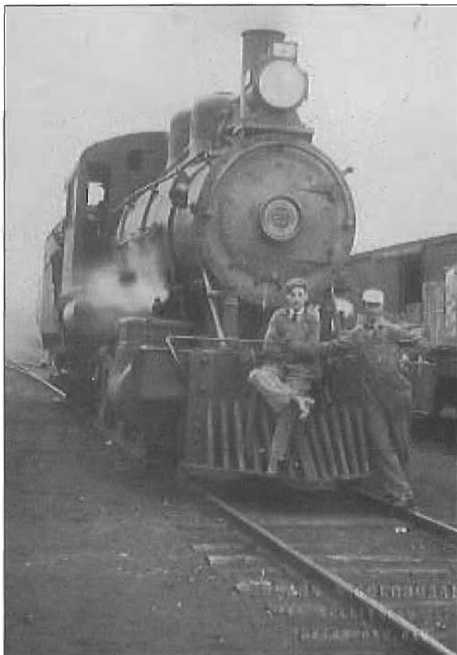
Three Quebec Central Railway photos, the first QCR locomotive No. 27 a 2-6-0 built by Canadian Locomotive Company in Kingston, Ontario. It operated on the QCR until 1939. Photo Derek Booth Collection.
