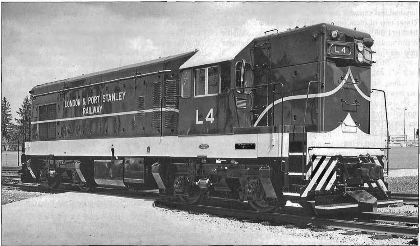
The L&PS's first diesel, a G12 export model purchased new from GMD London. The unit was delivered in August 1955, builders No. A831, it became CNR No. 991 on January 1, 1966. Photo courtesy GMD.
