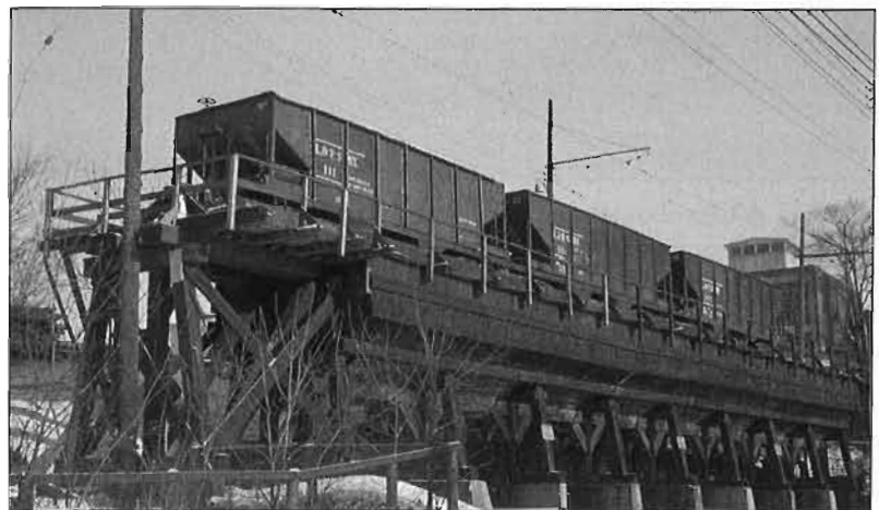
The very westerly extremity of L&PS electrified trackage in London was the coal yard at Bathurst Street west of the station. Here are three of the 50 ton, 2 bay coal hoppers owned by the L&PS, Nos. 110, 104 and 103. These were acquired in 1955 and used until 1966, the photo was taken on December 30, 1956.
