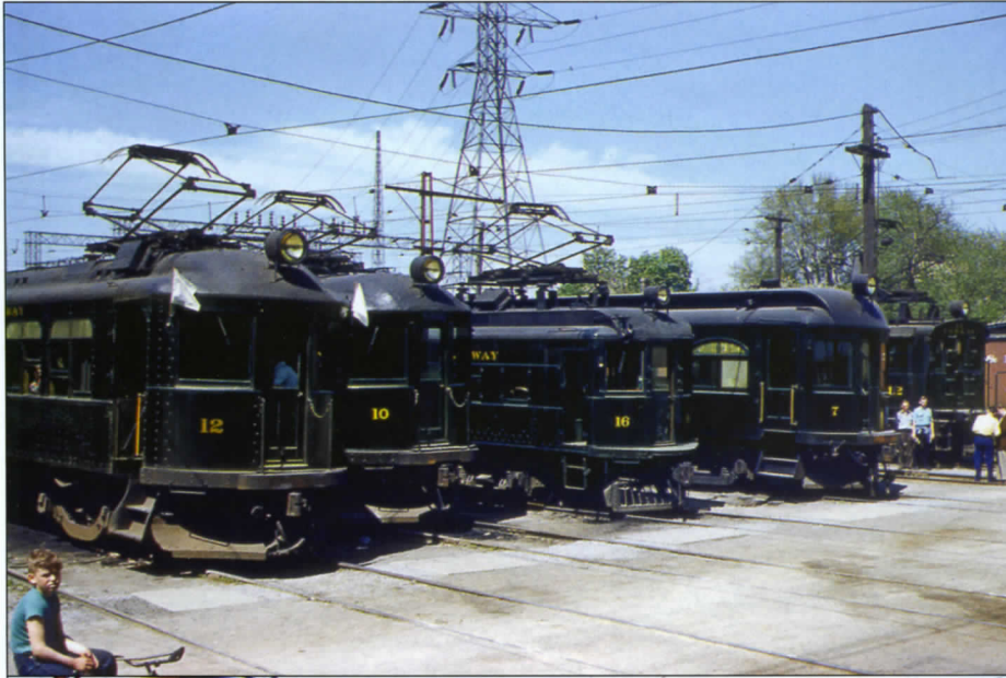
Most latter-day L&PS passenger stock types are represented in this portrait. From left to right are: Jewitt cars 12 (1917) and 10 (1915), Kuhlman 16 (1909), Preston trailer 7 (1915), CGE locomotive L2 (1915) and caboose C2 (1915 second hand). The photo was taken at the Philip Street shops in London on May 16, 1954.
