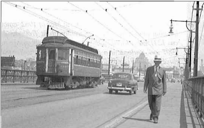
Car 1207 is a 1905 product of the British Columbia Railway's own shops, it is 50' 4" long and weights 71,550 Lbs. It is pictured here crossing the old Granville Street bridge bound for Marpole, the Hotel Vancouver is in the background. Car 1207 was restored by BC Transit at its Port Coquitlam bus depot and is presently in operation on the Downtown Historic Railway in Vancouver where it initiated service in 1998. Photo Stan Styles, GTC Collectibles
