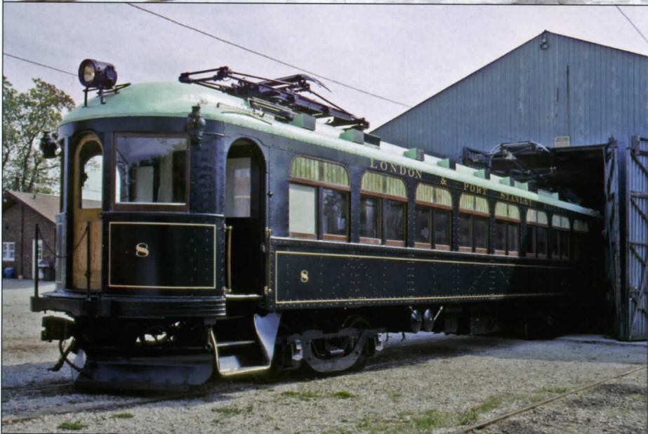
Car 8 was restored to resemble its original appearance by the Ontario Electric Railway Historical Association and shown here at the Halton County Railway Museum on August 27, 2000. The light-coloured roof reflects an early version which was eye-catching but did not last. Car 8 experienced a disastrous fire in the mid-1950's and the rebuilt version had the upper sash windows covered over. The OERHA included ne leaded windows in its restoration.
