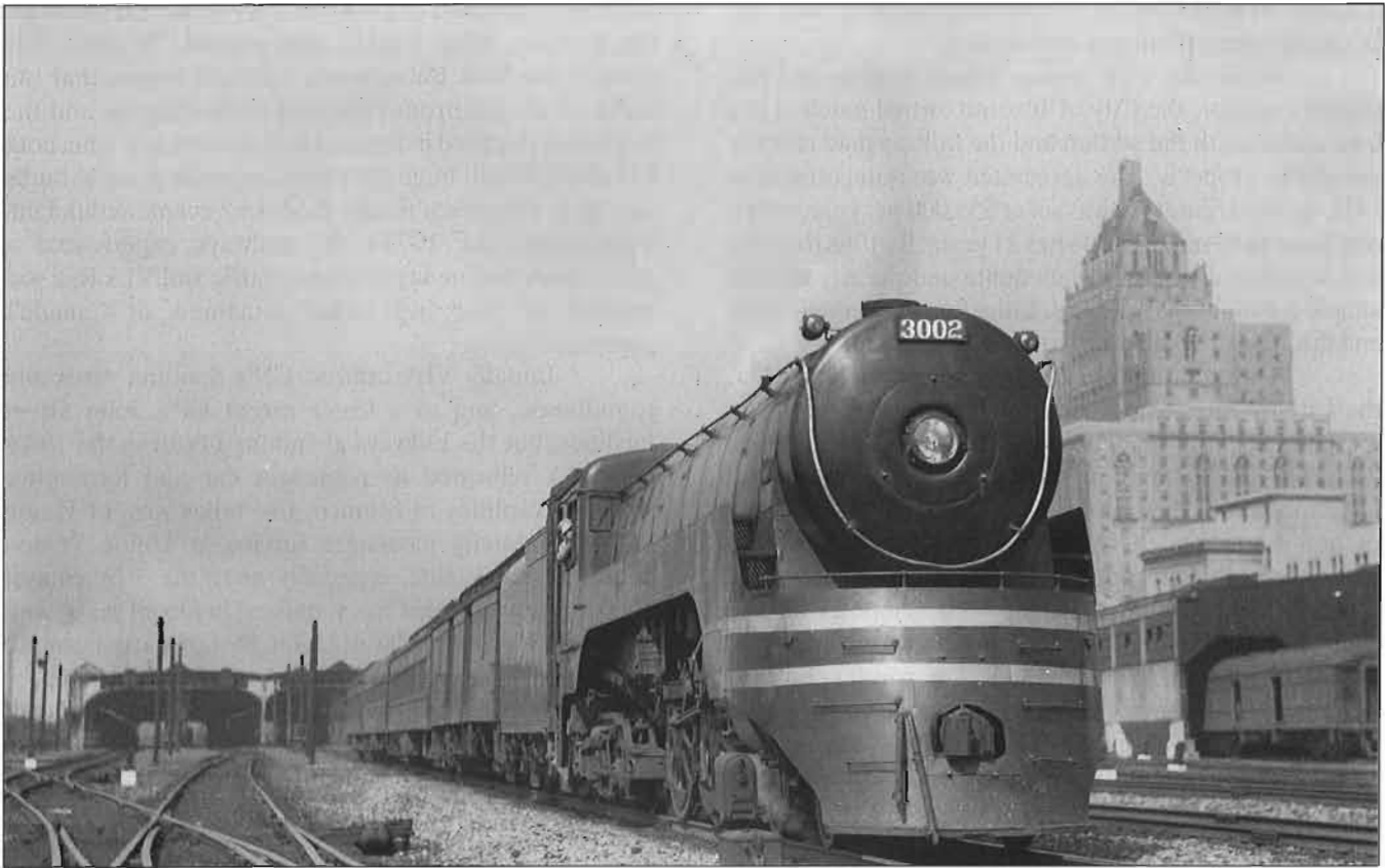
Canadian Pacific Train 36 departs from Union Station circa 1948, hauled by F2a 4-4-4 No. 3002. This was an all-stops local that took over ten hours to cover the distance between Toronto and Montreal. A heavyweight buffet-parlor car brought up the rear. Al Paterson photograph
