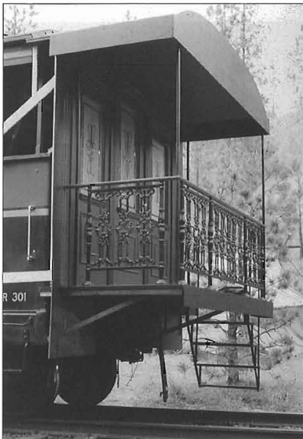
Details of a balcony end showing how it covers the coach's coupler. In real life this is KHR's open car, #301.
