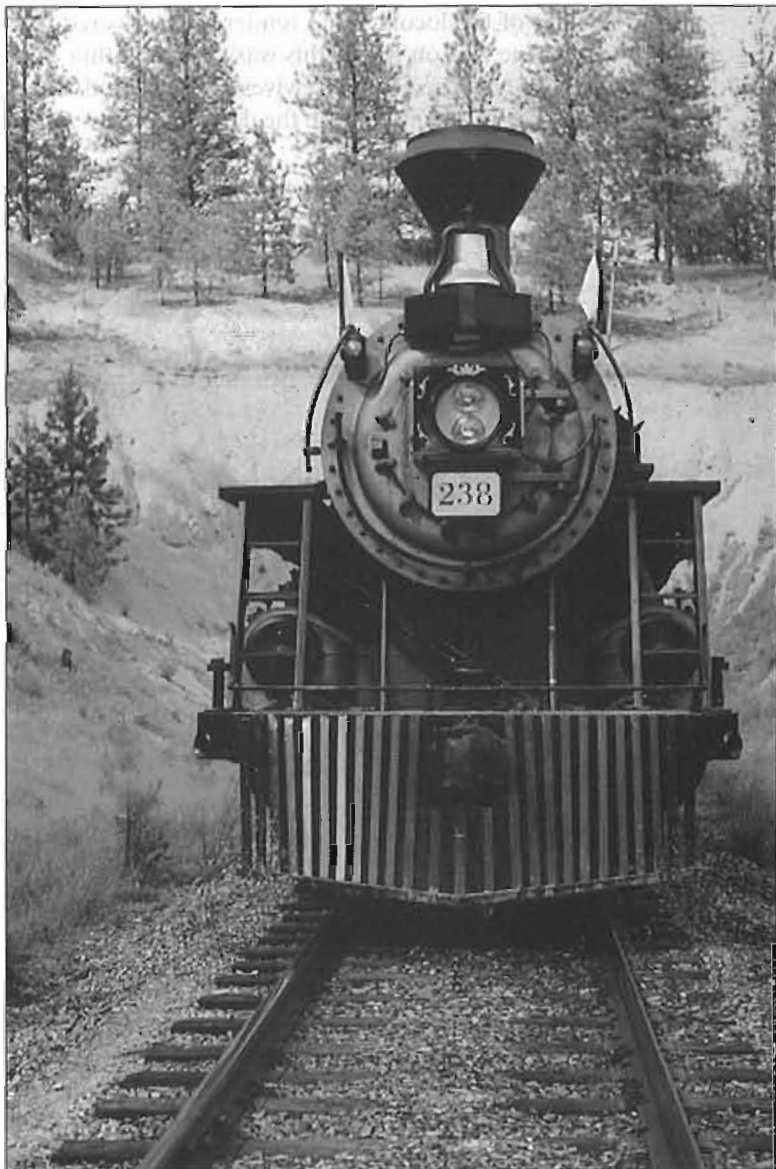
KHR loco 2141 fitted with balloon stack and cowcatcher; so as to become CPR #238.
