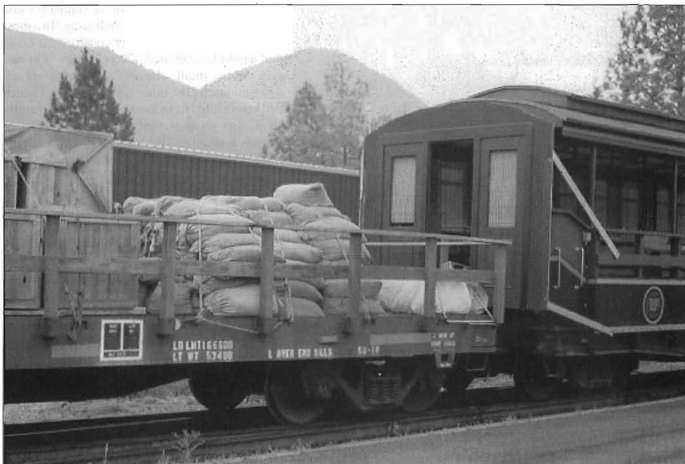
A modified open car viewed from its unchanged south side, together with rented flatcar carrying construction materials as seen in Kamloops interchange yard in early June 2007.
