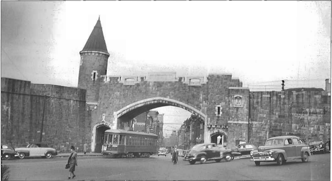
Car #610 can be seen passing through the St. Louis Gate on October 4, 1947. This car was one of five (610-614) built by the Ottawa Car Company in 1920 as a two-man car but later rebuilt by the QRL&P as a one-man car. Omer Lavallee, Ronald S. Ritchie Collection.
