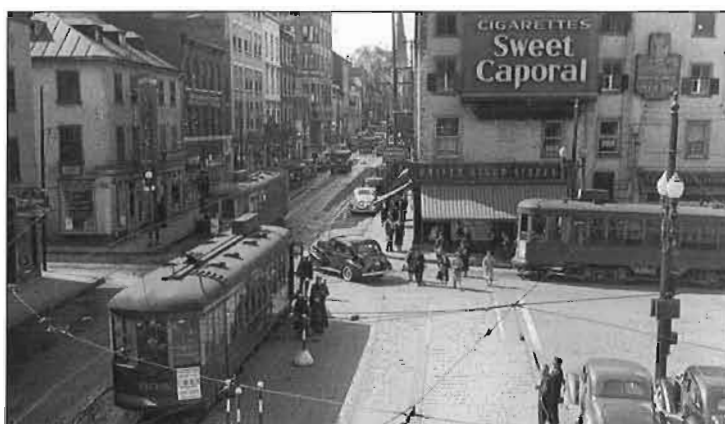
Car #805 is awaiting passengers in this c.1937 view at Place d'Youville in Upper Town at the intersection of St. John and d'Youville Sts. Note the QRL&P inspector on the sidewalk to the right, conversing with a gentleman. The 800 series steel cars (800-819) were built for the QRL&P by the Ottawa Car Company in 1928 and operated for 20 years when they were then retired. Al Paterson Collection.
