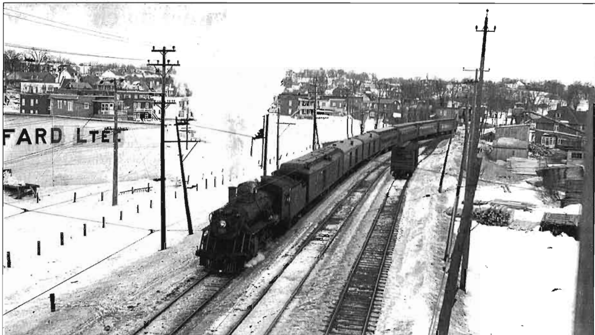
CNR Train 176 is in the charge of 4-6-0 1397 leaving Giffard for Murray Bay in this circa 1950 view. CNR power is running through from Quebec to Murray Bay obviating the need for an engine change from electric to steam at St. Joachim. Ronald S. Ritchie.
